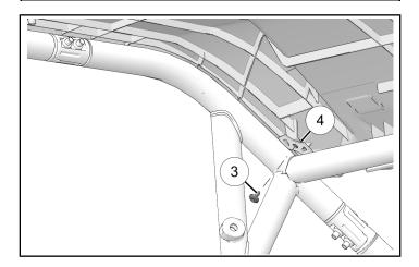
7. Install roof panel to roll-cage with two clamp assemblies.
