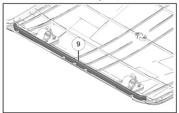
5. Put roof panel ① on top of roll-cage.
