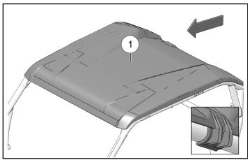
6. Install roof panel to roll-cage with two fasteners ③ installing into U-nuts ④ (previously installed).
