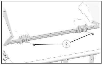
9. Torque two roof fasteners 3 to specification.
