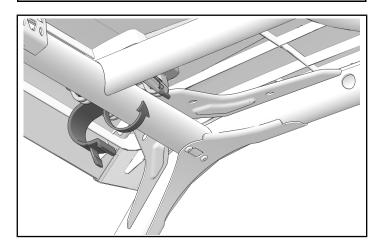
8. Install rear of roof panel with two fasteners ②. Torque fasteners to specification.
