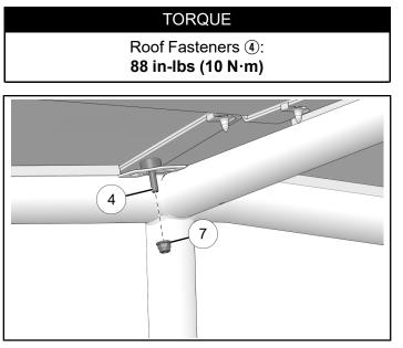
9. Torque six roof fasteners (9) to specification.
