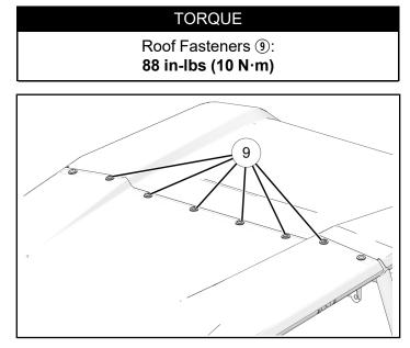
10. Torque front and rear roof fasteners 0 to specification.
