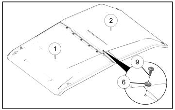
Install four cap inserts (1) and four rubber spacers (1) into front and rear roof panels. Push cap insert until it engages underside of roof.
