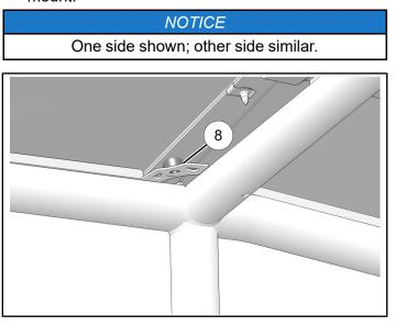
7. Put two screws ④ and two conical washers ⑥ through roof and previously installed spacer.
