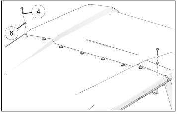
8. Install two nuts onto previously installed screws ④. Counter-hold nuts and two screws to specification.
