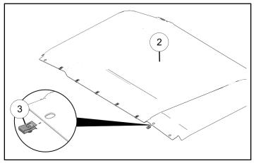
2. Put front roof panel ① over rear roof panel ② and loosely install with six screws ⑨ and six conical washers ⑥.
