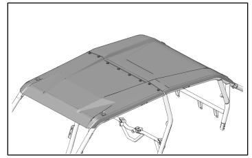
5. Loosely install roof panel to roll-cage with four fasteners (1) and four washers (5).
