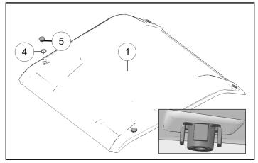
2. Put roof panel 1 on top of roll-cage.
