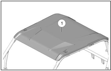
3. Loosely install roof panel to roll-cage with four fasteners ③ and four washers ②.
