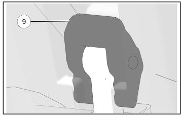
Install the body and lever assembly onto the vehicle cargo box using pin and push nuts to attach body and lever assembly to underside of cargo bed.
