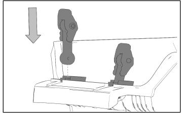
5. Install cover assembly using eight cover assembly screws ① into holes drilled into the cargo box.
