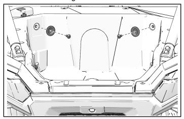
2. Remove and keep two screws from back of cargo box.
