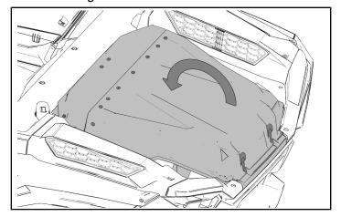
Loosely install stepped washers and attach to cargo box with two screws. Torque screws to specification.
