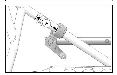
10. Torque all pivot bracket fasteners (5) to specification.
