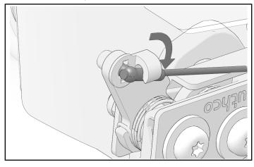
3. Remove and keep two screws, washers and nuts. Discard latch.
