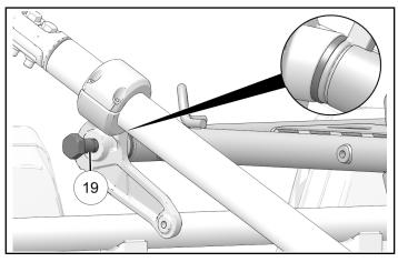
9. Measure distance between clamp assembly and top edge of roll cage joint. Make adjustments as needed.
