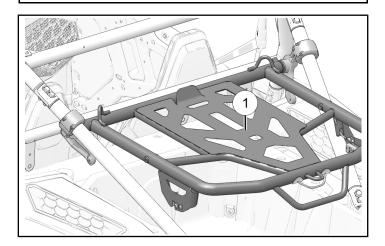
7. Push pivot brackets against tire rack and install pivot pins by hand.
