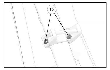
6. After adjustments are made, torque latch fasteners to specification.
