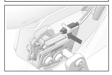
2. Rotate actuator cable out of clip and remove from latch assembly.
