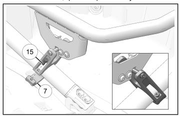
14. Make sure latch is perpendicular to striker. Adjust striker assembly on roll cage as needed.
