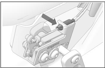
4. When tire rack is lowered, latches should hit strikers simultaneously.
