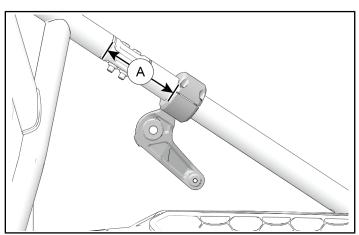
4. Measure distance between left and right clamp assemblies. Make adjustments as needed.
