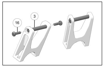
13. Install striker brackets with striker clamps ① and two fasteners ⓑ per clamp assembly.
