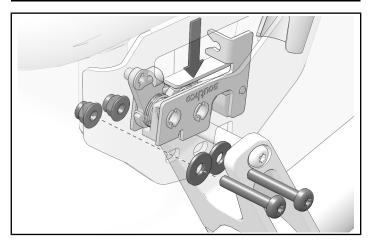
2. Put end of actuator cable into bracket slot and rotate cable into clip.
