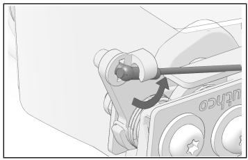
3. Push actuator cable into notch of latch bracket.
