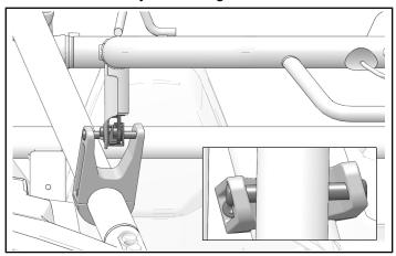
15. Measure distance between pivot clamp assembly and striker clamp assembly. Make adjustments as needed.
