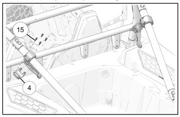
3. Measure distance between clamp assembly and top edge of roll cage joint. Make adjustments as needed.
