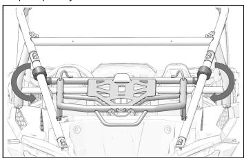
8. Continue to install pivot pins (9). Torque pivot pins to specification.
