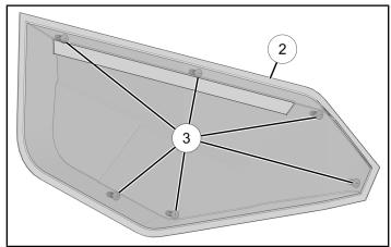
2. Identify six mounting holes in door frame.
