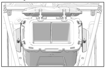
5. Push down on bracket to make sure it is flush against cargo box and close each Lock & Ride® lever to complete installation.
