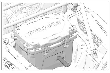
3. Lock & Ride® anchors may need adjustment. Tighten or loosen bottom nut depending on fitment.
