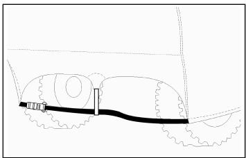
5. Ensure rear strap is positioned below lower rear tire lugs before strap is pulled taut by ratchet.
