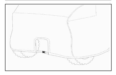
4. Route strap through rear center loop. Insert strap into partially closed ratchet and begin to operate ratchet mechanism.
