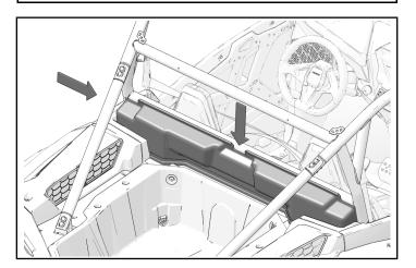
2. Put upper rear panel over lower rear panel and tilt top edge so that it rests on the inside of the upper cross-beam.
