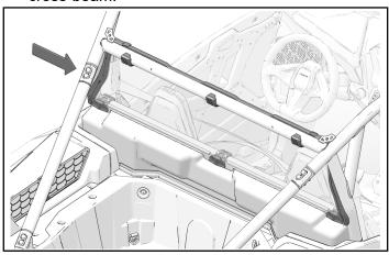
3. Upper rear panel should rest on the outside of the lower rear panel.
