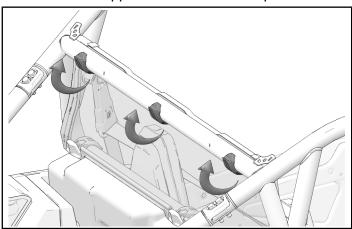
5. Push down on bottom rear panel and close three Lock & Ride® clamps.
