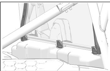
4. Top seal should rest on the inside of the upper cross-beam
