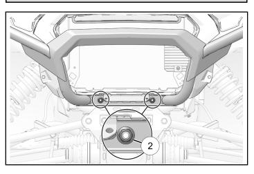
3. Install sides of front bumper with one nut (2) and one fastener (3) per side. Counter-hold nuts and torque fasteners to specification.
