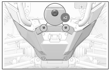
2. Remove two lower winch cover fasteners.
