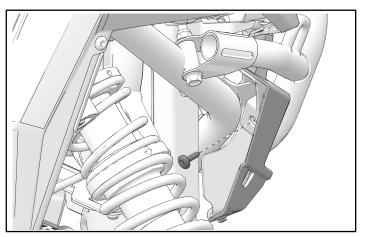
2. Remove one push-pin rivet from each side of front fascia.
