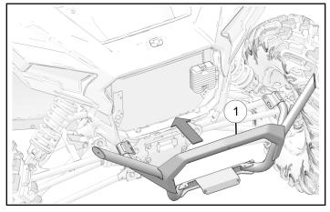
2. Loosely install front of bumper with two nuts 2.
