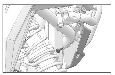
Install front fascia to radiator shroud with two push-pin rivets.
