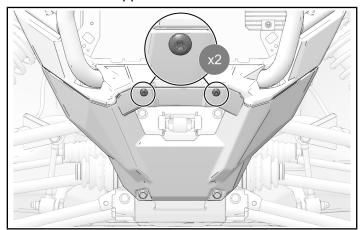
2. Remove two lower winch cover fasteners.
