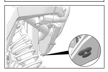
2. Remove two lower fascia fasteners.
