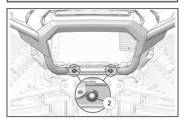
3. Install sides of front bumper with one nut ② and one fastener ③ per side. Counter-hold nuts and torque fasteners to specification.
