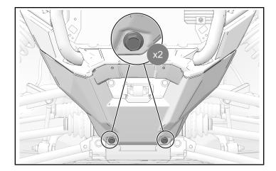
3. Install winch cover with two retained fasteners. Torque fasteners to specification.
