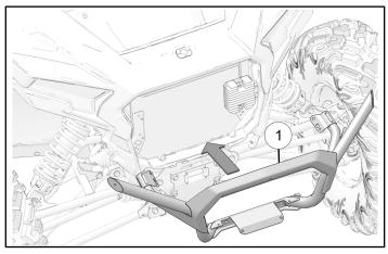
2. Loosely install front of bumper with two nuts ②.
