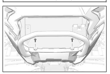
2. Install two upper fascia fasteners. Torque fasteners to specification.
