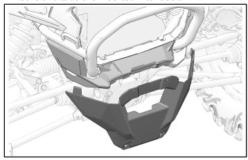
2. Install winch cover with two retained fasteners. Torque fasteners to specification.
