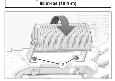
5. Torque light bar end nuts to specification.
