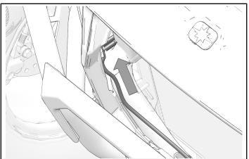
Connect two bullet connectors to corresponding connectors of light bar dashboard harness (sold separately). Use a cable tie (5) (not shown) to install harness to chassis.
