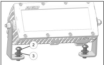
4. Align light bar assembly with drilled holes in front fascia panel and install to accessory bumper weld nuts. Torque two bolts ② to specification.
