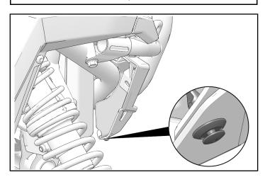
3. Install two upper fascia fasteners. Torque fasteners to specification.
