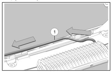
2. Put two bullet connectors through opening in radiator shroud.
