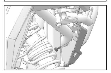
2. Remove one push-pin rivet from each side of front fascia.
