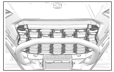
5. Put light bar connector through a hole in grille and connect to the back of the light bar.
