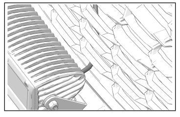
6. Put bottom of grille in first and push top of grille in until two tabs engage with upper front fascia.
