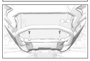
2. Install front fascia to radiator shroud with two push-pin rivets.
