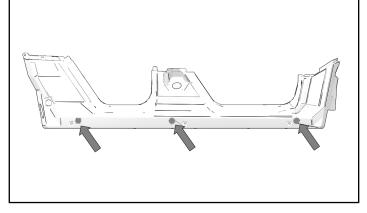
1. Find and mark the centers of the holes that are needed for the kit you are installing.
