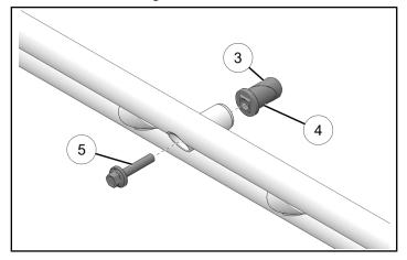
3. Tighten screw (5) until wedge anchor can barely move in all directions.
