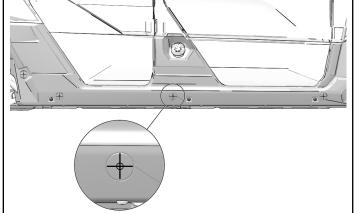
2. Drill a pilot hole at the center of each hole.
