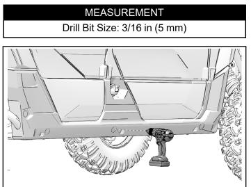
3. Cut each desired hole with hole saw.
