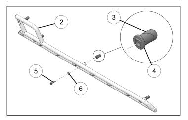
Screw (5) will pass through unthreaded wedge lock anchor (4) and thread into threaded wedge lock anchor (3). Note orientation of wedge anchor. Anchor will expand in the forward/backward direction when tightened.
