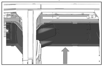
6. Install nine screws to hold mid roof liner to roof.
