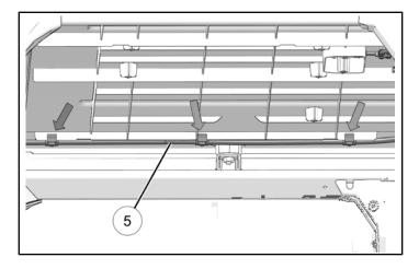
4. In rear seat compartment, clip harness ③ to rear of roof at points shown.
