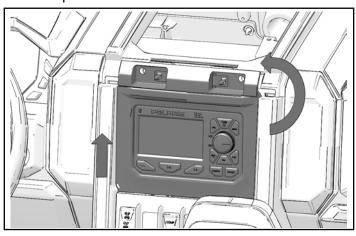
3. Disconnect wiring harness and antenna from head unit. Remove head unit.
