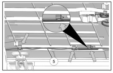
8. In cargo compartment, clip harness ⑤ to rear of roof at points shown.
