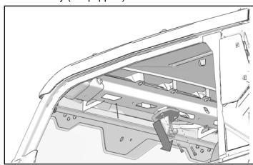
2. Remove and keep six screws from top of roof liner and four screws from front of roof liner.
