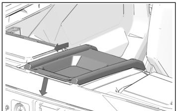
2. Install two push-pin rivets.
