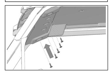
14. Connect dome light ② to connector on harness ⑤. Repeat for other dome light.
