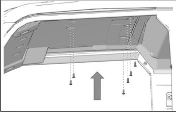
13. Install five screws in front edge of roof liner. Torque screws to specification.
