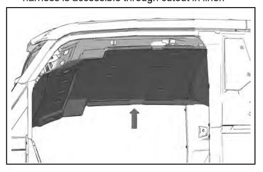
4. Install six screws to hold roof liner to roof. Torque screws to specification.
