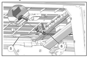
2. Route harness (6) along right side of roof. Clip harness to roof of cargo area at points shown.
