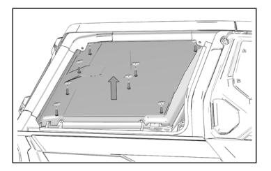
11. Install front roof liner. Make sure dome light harness is accessible through cutout in liner.
