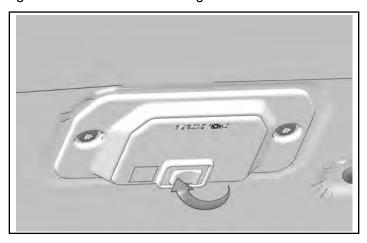
Press driver side of dome light switch to turn off dome light.
