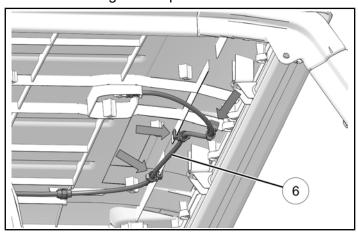
4. Install rear roof liner. Make sure dome light harness is accessible through cutout in liner.
