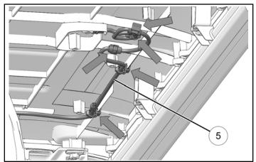
9. Install rear roof liner. Make sure dome light harness is accessible through cutout in liner.
