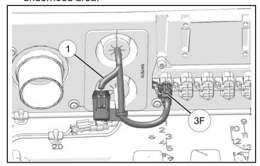
2. Connect harness ① to ROPS harness. Insert connector into the appropriate connector on ROPS harness. Use cable tie on harness to attach harness to chassis at point shown.
