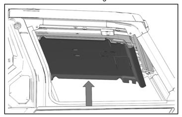
5. Install eight screws to hold rear roof liner to roof. Tighten screws to specification.
