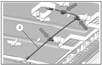
3. Install front roof liner. Make sure dome light harness is accessible through cutout in liner.
