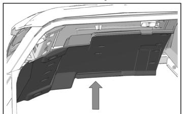
12. Install six screws to hold roof liner to roof. Torque screws to specification.
