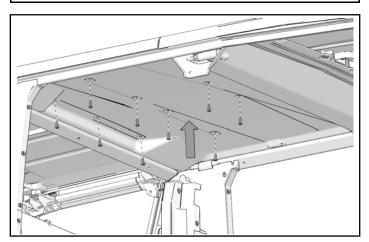
7. In cargo compartment, clip harness ⑤ to right side of roof at points shown.
