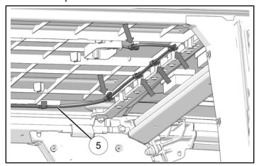
5. Install mid roof liner. Make sure dome light harness is accessible through cutout in liner.
