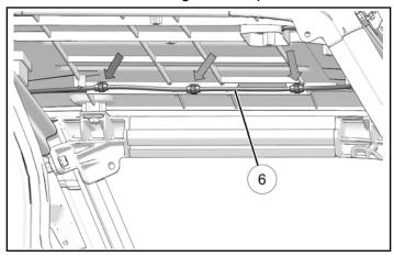
3. Route harness ⑥ across rear of roof. Clip harness to roof of cargo are at points shown.
