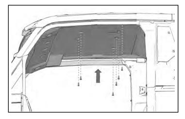
5. Install five screws in front edge of roof liner. Torque screws to specification.
