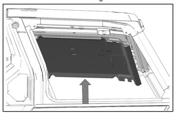
10. Install eight screws to hold rear roof liner to roof. Torque screws to specification.
