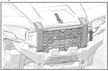
3. Pull rubber straps off hooks to release hood. Lift hood to remove.
