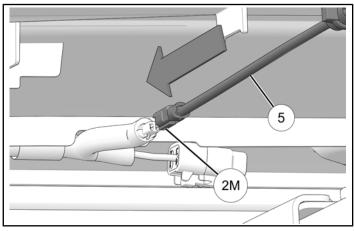
2. Clip harness ⑤ to roof at points shown. Route remaining leg of harness over ROPS, into rear compartment. as shown.
