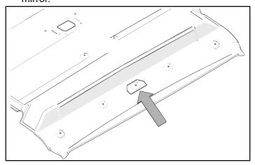
3. Install speed nuts ② into the openings in the ROPS.
