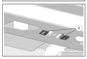
4. Reinstall roof line using kept screws. Torque screws to specification.
