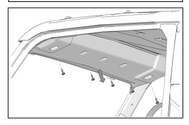
2. Lower the front of the roof liner. Cut along the existing trim line to create the opening for the mirror.
