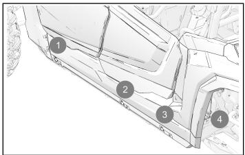
4. Align rock slider with rear mounting location first and then swing the rock slider towards the vehicle to align the final three mounting locations.
