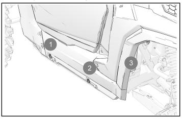
3. Align rock slider with rear mounting location first and then swing the rock slider towards the vehicle to align the final two mounting locations.
