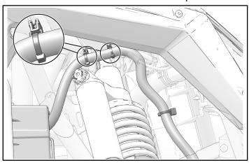
4. Identify four mounting locations for contactor box.
