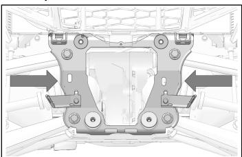
3. Mount winch onto vehicle with two hooks. Install winch with four fasteners ®. Torque fasteners to specification.
