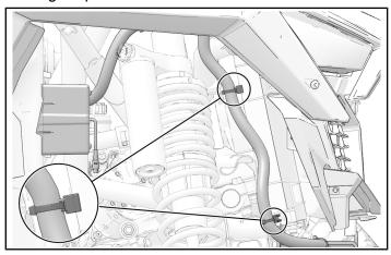
3. Install winch harness to chassis, above right-hand suspension, with edge clips. Use cable ties ⑤ (not shown) to install excess winch harness to chassis and to make sure it is clear of the suspension.
