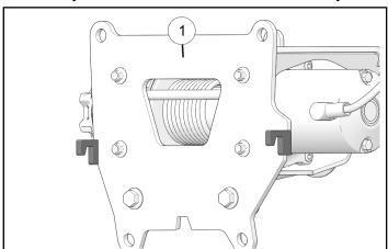
2. Identify two slots on vehicle chassis.
