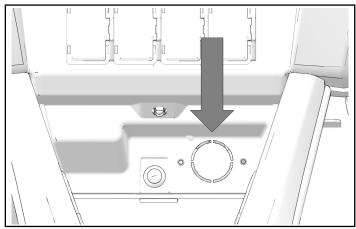
2. Install winch remote socket ③ with two remote socket fasteners ⑥. Torque fasteners until fully seated.
