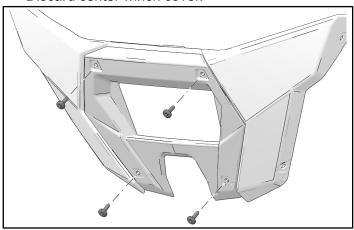
2. Install new winch cover ④ with four retained fasteners.
