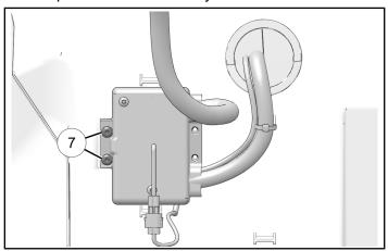
6. Install two screws ① until fully seated.
