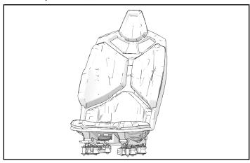
Tilt seat assembly forward and pull back slightly to disengage from receiver tube and remove seat from vehicle.
