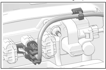
9. Do not remove existing nuts from negative and positive terminals. Install negative (black) and positive (red) terminal rings with two nuts (9).
