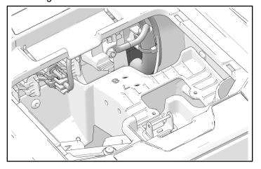
8. Install winch harness to Polaris Pulse® bar. Install excess harness to firewall with edge clip.
