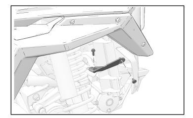
2. Install winch harness along radiator shroud with edge clips.
