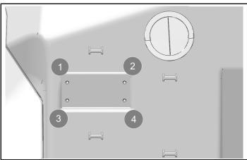
5. Install contactor box with two outside screws ①. Torque fasteners until fully seated.
