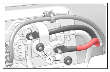
Reinstall fascia bracket in front of winch harness with two retained fasteners. Torque fasteners to specification.
