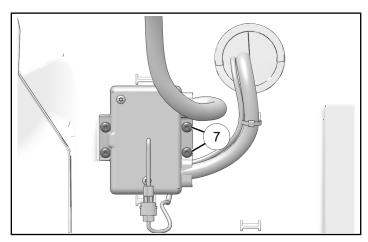
7. Put winch harness, extending from contactor box, through firewall hole and into under-dashboard.
