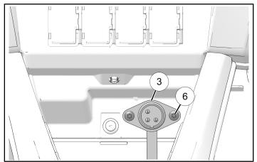
3. Connect remote socket connector ③ to winch remote connector.
