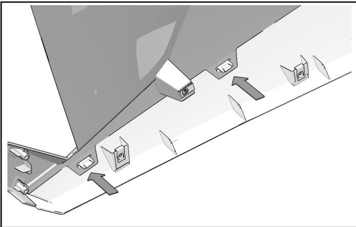
7. Align door panel with door frame and install with eleven (11) retained door panel fasteners.
