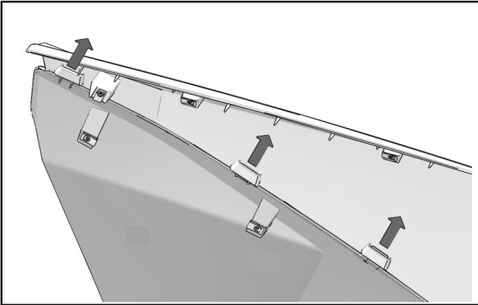
6. Slide close-off panel over bottom tabs protruding from door panel.
