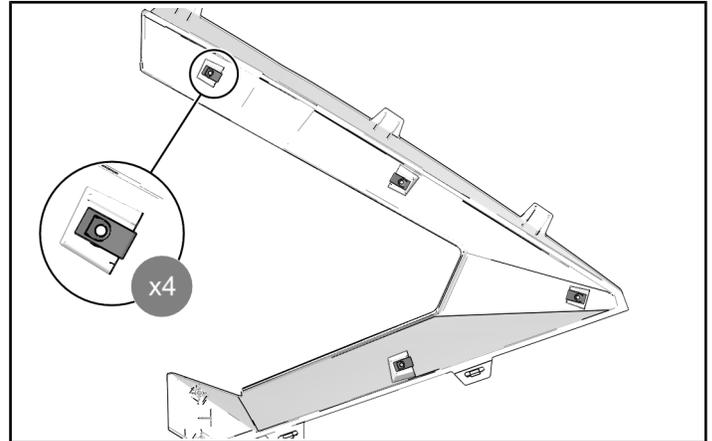
3. Install four retained U-nuts to mounting locations of accessory close-off panel.
