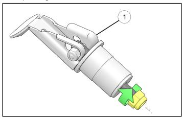
4. With brackets and anchors aligned, close each Lock & Ride® clamp.
