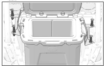
3. Lock & Ride® assemblies ① may need adjustment. Tighten or loosen bottom nut depending on fitment.
