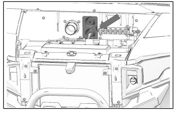
5. Install upper center dash panel. Engage rear tabs into slots, then lower front of panel into place Install two push darts.
