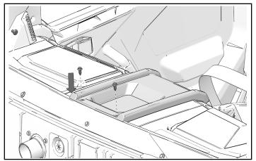
6. Install base (5), three screws (13), and three washers (15).
