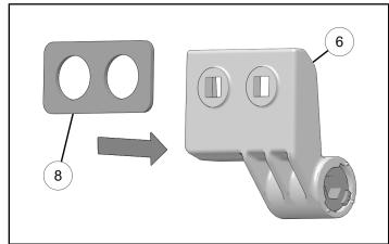
8. Attach mount (6) to windshield assembly (2). Push mount fully into hinge.
