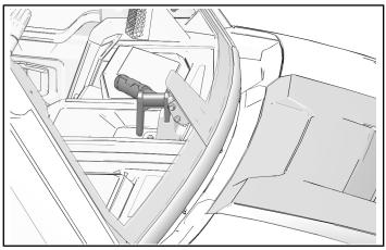
11. Insert carriage bolts (1) through the mounts and the mounting holes.
