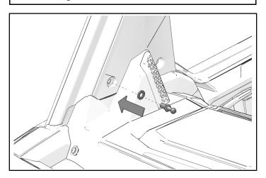
2. Install bracket ① through the opening that was covered by the upper center dash panel. Line up mounting holes with the holes in the frame.
