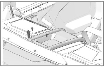
2. Turn over upper center dash panel. Locate three divots on the underside of the panel. Drill holes at these locations.
