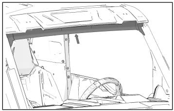
Remove backing paper and install windshield seal
