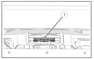
3. Install screws (1). Access screw holes through the opening where the grommet was removed. Torque to specification.
