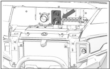
4. Remove frontmost screw from each inside sail panel.
