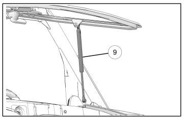
14. Adjust base to achieve desired seal pressure at bottom of windshield. When adjustment is complete, torque base screws to specification.
