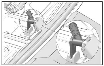
• Disengage the handle from the base to put the windshield in the fully open position.
