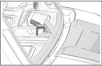
• Place the handle in the position shown to put the windshield in the vented position.
