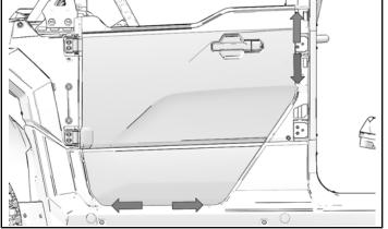
2. After door is properly positioned, check engagement with striker. Adjust striker up or down as needed for proper latching. If door does not seal or rattles when latched, adjust striker inward. If door is difficult to open, adjust striker outward. Remove striker cover to access striker screws.
