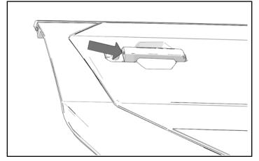
4. Lift handle away from actuator and pull backwards to remove handle. Keep handle for later installation.
