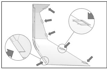
3. Filler panel for 2-passenger doors has seven engagement points. Lower rear corner of panel fits over a tab on door, and there is one tab that will fit into a slot on door. Five other tabs engage with main trim panel on door.
