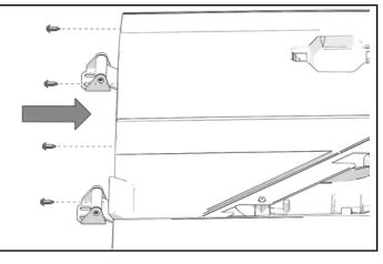
5. Lower previously removed filler panel and slide forward into proper position.
