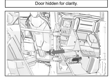
2. Remove two screws and limit strap bracket from rear of B-pillar.
