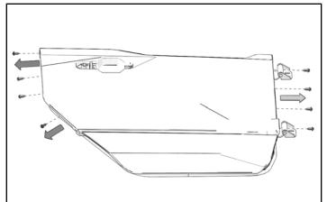
6. Move panel toward rear and lift to remove panel. Keep panel for later installation.
