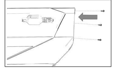
7. Install previously removed door handle through opening in panel.
