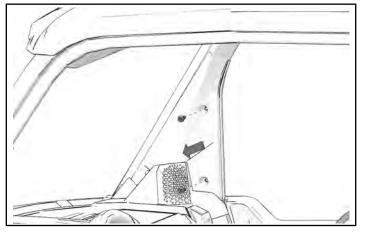
4. Pull panel outward and pull toward front of vehicle to remove panel.
