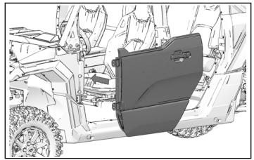
2. Loosely install four hinge screws.
