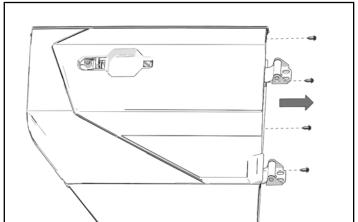
6. Remove and keep three push pin rivets from rear of door.
