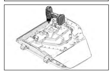
3. Turn door over. Mount clamps to the inside surface of the door. Tighten screws to specification.
