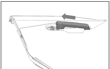
5. Remove and keep eight push pin rivets from door.
