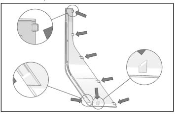
4. Front door has five slots along top and five slots along bottom. Tabs from trim panels fit into these slots. Additionally, there is a tab at lower rear of door which engages a slot on trim panels.
