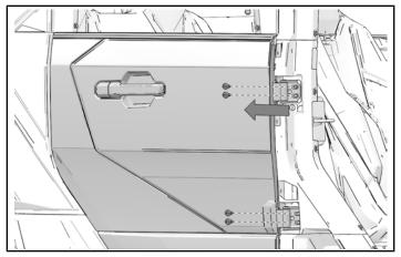
5. Pull door handle to disengage striker and lift door away from vehicle.
