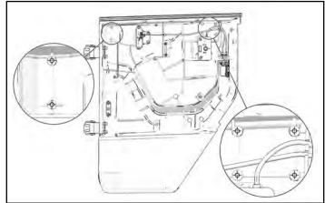
2. Drill through the center of each boss. Drill through the inside surface of the door.
