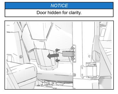
3. Close door and engage door with striker. This will help support door while hinge screws are removed.
