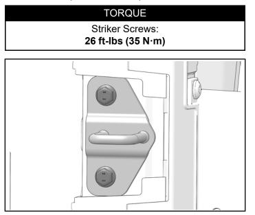
4. Thread bracket through limit strap. Install bracket and two screws to A-pillar. Torque bracket screws to specification.
