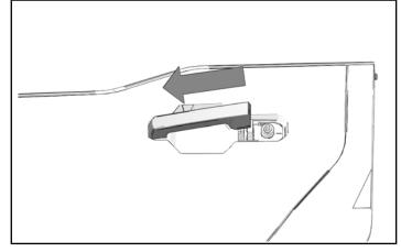
8. Handle must engage hinge under panel for handle to work properly, Handle will audibly click into place on loop.
