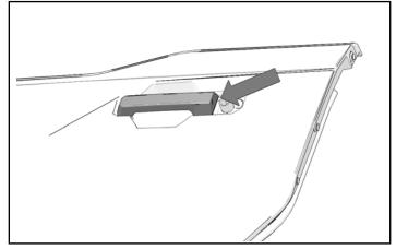
7. Push previously removed cover into place over actuator.
