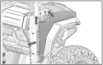
2. Remove and keep two screws from front fender.
