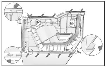
Rear door has three slots along top and one slot at bottom. Tabs from trim panels fit into these slots. Additionally, there is a tab at lower rear of door which engages a slot on trim panels.
