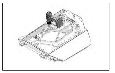
3. Turn door over. Mount clamps to the inside surface of the door. Tighten screws to specification.
