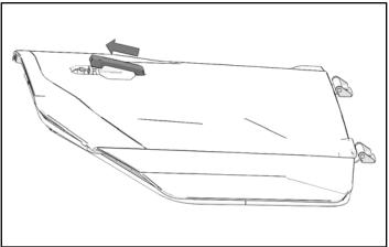
5. Remove and keep four push pin rivets from front of door.
