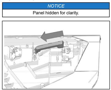
9. Lower handle over actuator. Install previously removed screw to attach handle to actuator.
