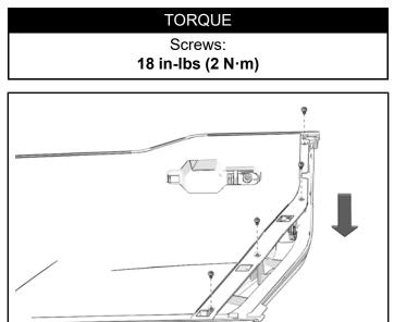
4. Install four previously removed push pin rivets.
