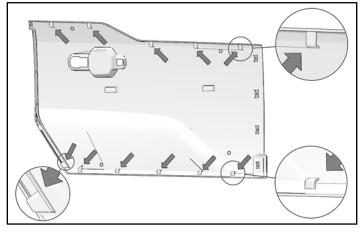
2. Filler panel for rear doors has six engagement points. Lower rear corner of panel fits over a tab on door. Five other tabs engage with main trim panel on door.
