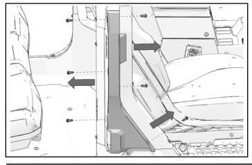
2. Turn top of trim away from vehicle. Lift trim to disengage the lower tab. Remove trim.
