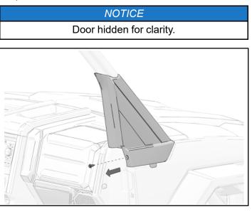
3. Remove and keep two screws from inner panel.
