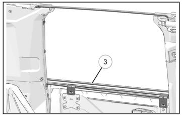
2. Install knobs (8) to attach frame (3) to clamps.
