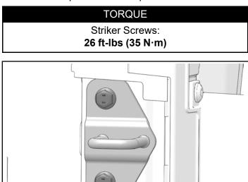
4. Thread bracket through limit strap. Install bracket and two screws to A-pillar. Torque bracket screws to specification.
