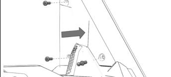
3. Return clip at bottom of gas spring to engaged position. Connect bottom of gas springs.
