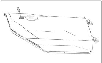
3. Remove and keep screw to separate handle from actuator.
