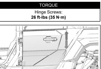
2. After door is properly positioned, check engagement with striker. Adjust striker up or down as needed for proper latching. If door does not seal or rattles when latched, adjust striker inward. If door is difficult to open, adjust striker outward. Remove striker cover to access striker screws.
