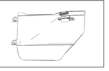
5. Handle must engage hinge under panel for handle to work properly. Handle will audibly click into place on loop.
