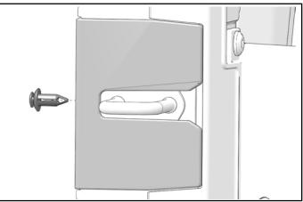
3. When finished adjusting striker, torque striker screws to specification. Replace cover.
