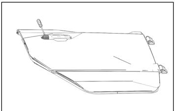
3. Remove and keep screw to separate handle from acuator.
