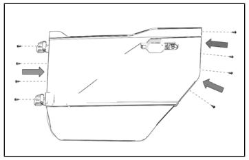
4. Install previously removed door handle through opening in panel.
