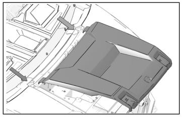
2. Pull rubber straps down over hooks to secure hood.
