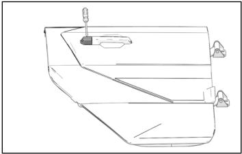
3. Remove and keep screw to separate handle from actuator.
