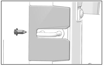
3. When finished adjusting striker, torque striker screws to specification. Replace cover.
