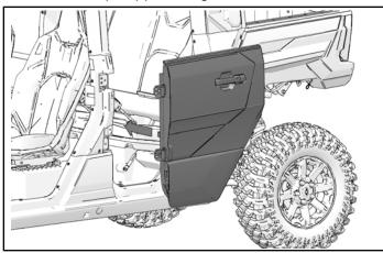
2. Loosely install four hinge screws.
