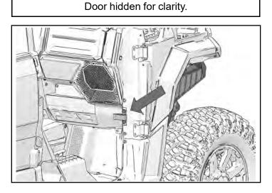
2. Remove two screws and limit strap bracket from A-pillar.
