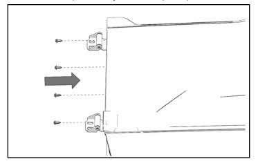
5. Lower previously removed filler panel and slide forward into proper position.
