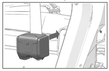
2. Install nut on rear of retractor. Torque nut to specification.
