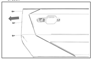
7. Move filler panel toward rear and lift to remove panel. Keep panel for later installation.
