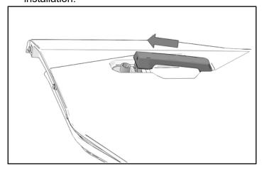
5. Remove and keep eight push pin rivets from door.
