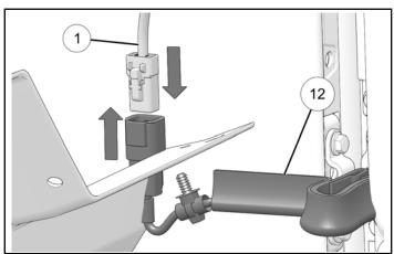
7. Install harness mount into hole in lower dashboard.
