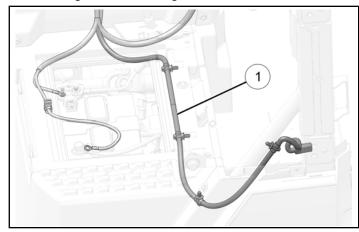
27. Route harness ① along rear side of battery box. Install two harness clips into holes in front side of rear seat base tube.
