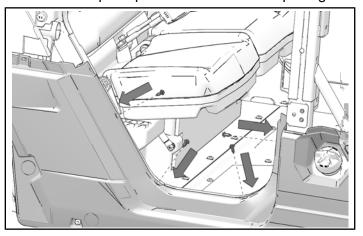
Pull out on bottom edge of rear fender. Install two push-pin rivets and one screw in top edge of bottom rocker panel. Torque screw to specification.
