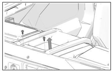
Remove and keep panel by lifting front edge and moving backward.
