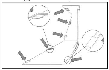
3. The front door has five slots along the top and five slots along the bottom. Tabs from the trim panels fit into these slots. Additionally, there is a tab at the lower rear of the door which engages a slot on the trim panels.
