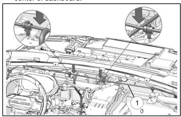
4. Continue routing right leg of harness ①. Install mounts into next routing clip and into hole in dashboard frame. Edge clip near harness end will attach to dashboard when dashboard is installed.
