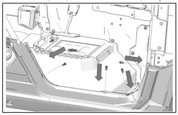
8. Install four push-pin rivets in rear door opening.
