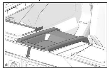
2. Install two push-pin rivets.
