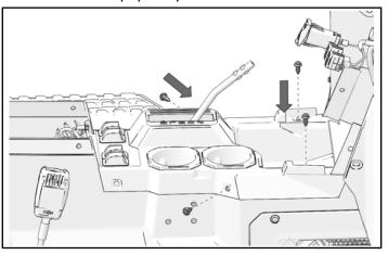
21. Install kept grab handle. Torque screws to specification.
