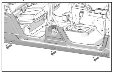
6. Remove and keep six screws from underside of bottom rocker panel.
