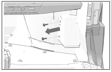
5. Remove and keep three screws from bottom rocker panel.
