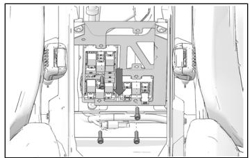
6. Remove four screws to disassemble bracket from center console.
