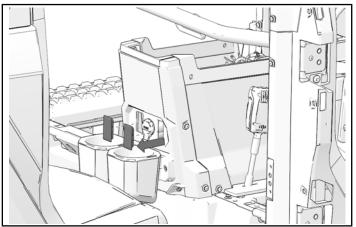
25. Connect two switches ⑤ to harness connectors. Push switches into openings in console until switches lock into place.
