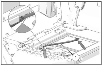
32. Detail view of harness routing near fuel tank,
