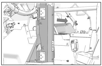
3. Remove and keep two push-pin rivets from inside of lower rocker panels.
