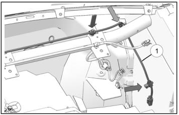
5. Route left leg of harness ①. Install mount into left side routing clip. Edge clip near harness end will attach to dashboard when dashboard is installed.
