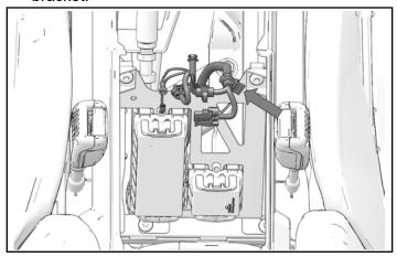
2. Remove covers from fuse boxes. Pull up on yellow handles on each end of fuse block.
