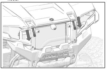
3. Put tabs on grill through openings in front fascia. Push top of grill into correct position.
