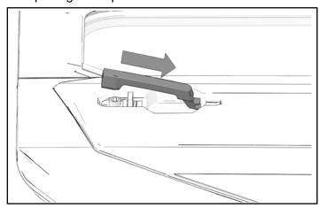
8. Handle must engage hinge under the panel for handle to work properly. Handle will attach to loop with audible click.
