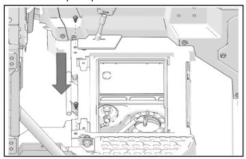
2. Push battery cover forward and lower into place.
