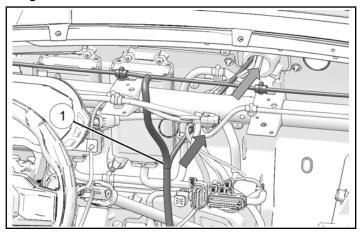
7. Connect front leg of harness ① to Polaris Pulse® Bar.
