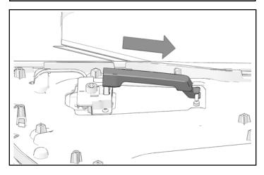
6. Lower handle over actuator. Install previously removed screw to attach handle to actuator.
