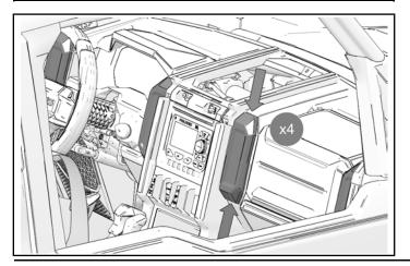
2. Remove one screw at each side of dash cover.
