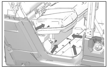
3. Remove and keep five push-pin rivets from front door opening.
