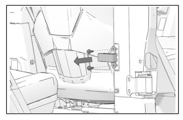
3. Close door and engage door with striker. This will help support door while hinge screws are removed.
