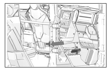
2. Remove two screws and limit strap bracket from rear of B-pillar.
