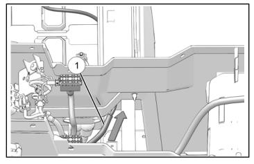
13. Left side view of battery harness routing. Note location of edge clip. Attach edge clip to underside of floor panel.
