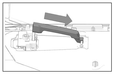
9. Lower handle over actuator. Install previously removed screw to attach handle to actuator.
