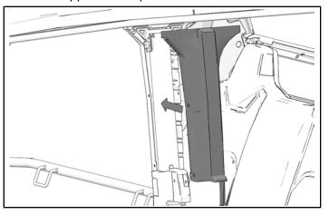
2. Install two screws in inside panel. Torque screws to specification.
