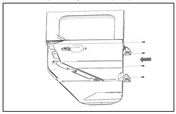
5. Lower previously removed filler panel and slide forward into the proper position.
