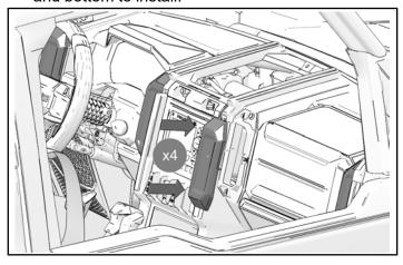
7. Install one push pin rivet at each side of dash.
