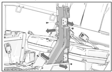
2. Remove and keep two push-pin rivets from rear side of lower rocker panel.
