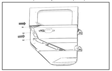
7. Install previously removed door handle through the opening in the panel.
