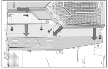
5. Remove push-pin rivet from bottom of dashboard in front of drivers seat.
