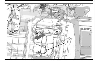
14. Connect terminal with black shrink wrap to negative battery terminal. Connect terminal with red shrink wrap to positive battery terminal. Install nut (6) at positive battery terminal. Torque nut for positive terminal to specification.
