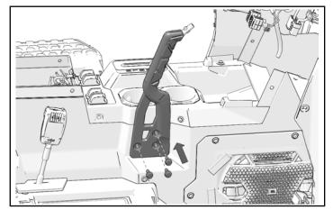
22. Install shift handle knob base. Torque kept screw to specification.
