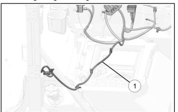
31. Route harness ① across top of fuel tank. Attach two harness edge clips to ribs on underside of right floor panel.
