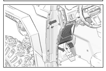
2. Carefully pull trim away from vehicle and remove one push-pin rivet from side of dashboard.
