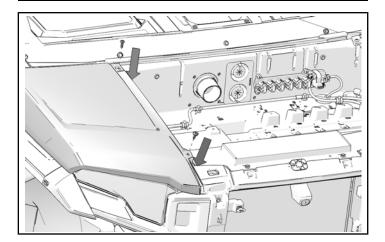
4. Install four push pin rivets.
