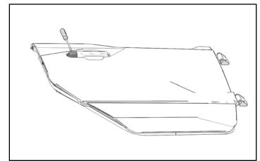
3. Remove and keep screw to separate handle from acuator.
