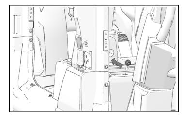
3. Install rubber plug behind seat belt retractor.
