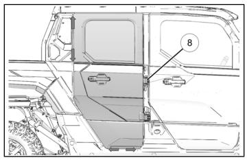
2. After door is properly positioned, check engagement with the striker. Adjust striker up or down as needed for proper latching. If door does not seal or rattles when latched, adjust striker inward. If door is diffcult to open, adjust striker outward. Remove striker cover to access striker screws.
