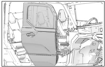
2. Loosely install four hinge screws 8.
