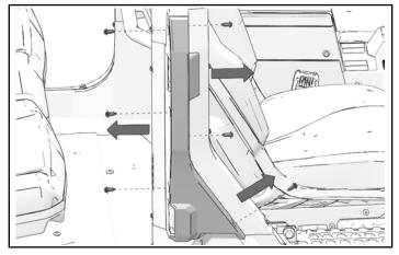
2. Turn top of trim away from vehicle. Lift trim to disengage the lower tab. Remove trim.
