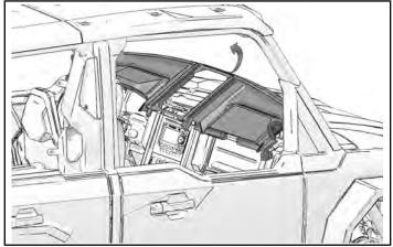
9. If vehicle is equipped with upper tweeters, make sure to unplug tweeters when removing dash cover.
