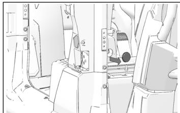
2. Remove and keep nut from rear of retractor.
