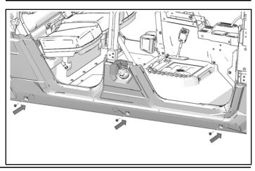
6. Install two screws in side of foothold in front of passenger seat area. Torque screws to specification.
