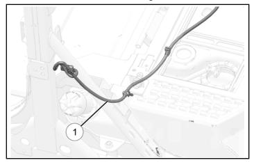
33. Route harness ① toward fuel filler tube. Attach harness clip into hole on rear side of seat base tube.
