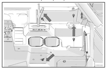
5. Place shift lever in NEUTRAL position. This will aid removal and later installation.
