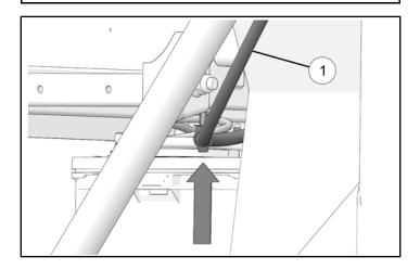
29. Route harness ① up rocker tube. Install harness clip into hole on underside of rocker tube.
