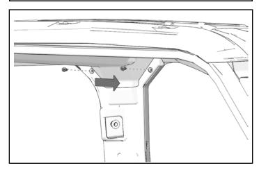
3. Install four push-pin rivets.
