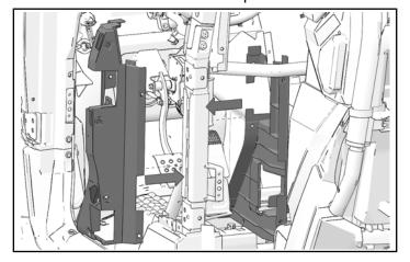
2. Install two push-pin rivets on inside of lower rocker panels.
