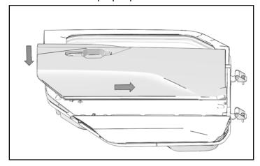
3. Install eight previously removed push pin rivets.
