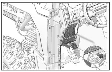
7. Install screw and push-pin rivet in left side door frame.
