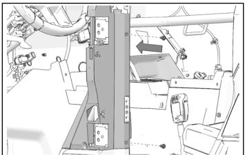
4. Install four push-pin rivets in lower rocker panels. Install one screw in lower rocker panel. Torque screw to specification.
