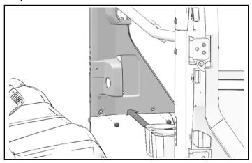
3. Install two push-pin rivets on rear side of lower rocker panels.
