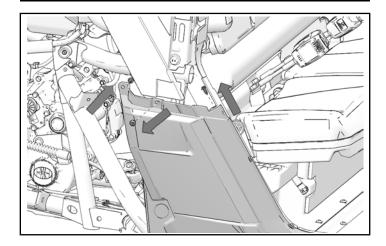
2. Remove and keep four push-pin rivets from rear door opening.
