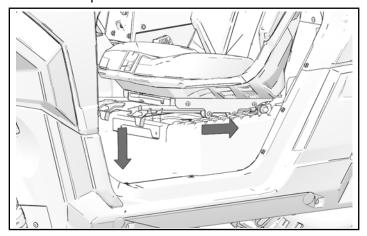
5. Install two kept screws at front of seat base. Torque screws to specification.
