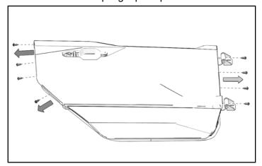
6. Move panel toward rear and lift to remove panel. Keep panel for later installation.
