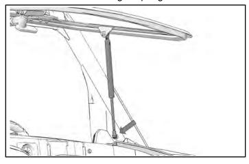
4. Remove two screws and ball stud from lower A-pillar trim panel.
