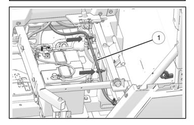
28. Continue to route harness ① along rear seat base tube. Install harness clip into hole in bottom of rear seat base tube.
