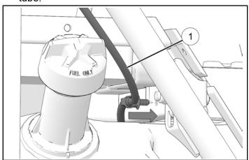
34. Route harness ① up rocker tube. Install harness clip into hole on underside of rocker tube.
