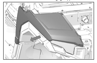
4. Turn fender and lift to disengage lower tab and remove fender.
