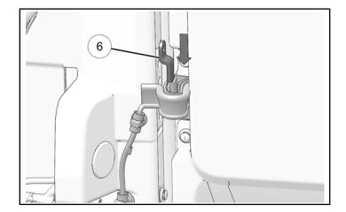
5. Install two screws ① to attach bracket ⑥ to A-pillar. Torque bracket screws to specification.
