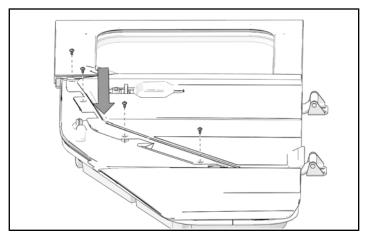
4. Install four previously removed push pin rivets.
