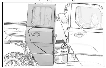
3. Loosely install four hinge screws ①.
