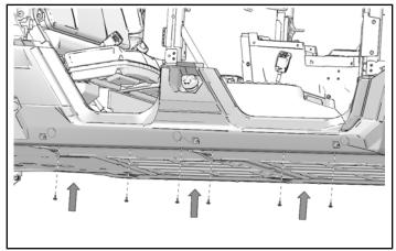
5. Install three screws in bottom rocker panel. Torque screws to specification.
