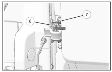
6. Install harness mounts into holes in B-pillar.
