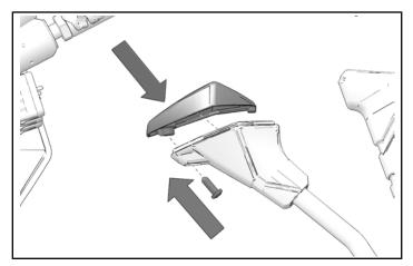
24. Remove two switch covers from rear of center console.
