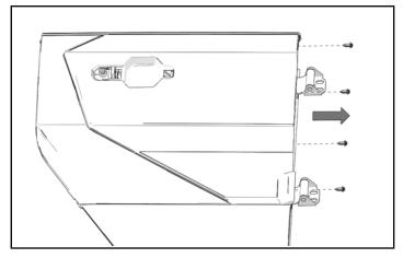
6. Remove and keep three push pin rivets from rear of door.
