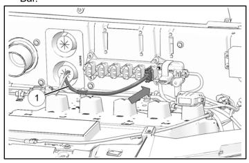
8. Route remaining harness leg down to center console area. Attach edge clip to grab handle mounting bracket.
