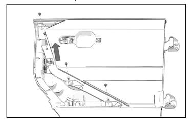
9. Move trim panel toward rear and lift to remove panel. Keep panel for later installation.
