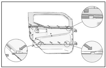
4. The rear door has five slots along the top and one slot at the bottom. Tabs from the trim panels fit into these slots. Additionally, there is a tab at the lower rear of the door which engages a slot on the trim panels.
