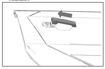
5. Remove and keep four push pin rivets from front of door.
