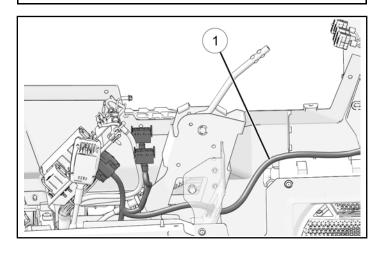
9. Remove cover from fuse block on harness ①.
