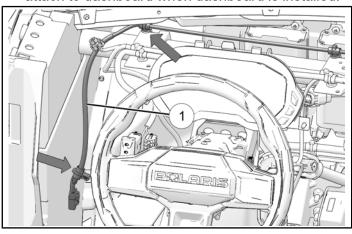
6. Route front leg of harness ① through lower grommet hole to underhood area.
