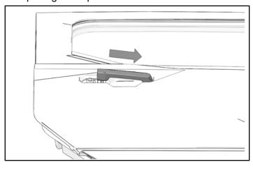
5. Handle must engage hinge under the panel for handle to work properly. Handle will attach to loop with audible click.
