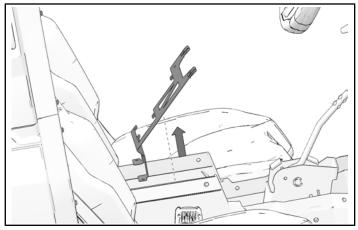
8. Install two U-clips (3) at top of bracket (4).
