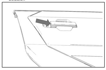
4. Lift handle away from actuator and pull backwards to remove handle. Keep handle for later installation.
