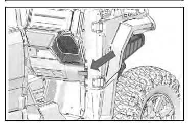
2. Remove two screws and limit strap bracket from A-pillar.
