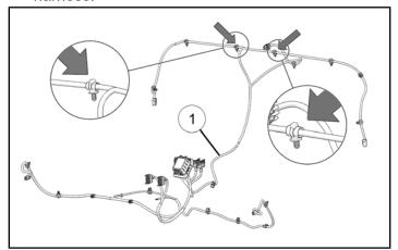
3. Install harness mounts into routing clips at top center of dashboard.
