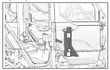
2. Place door in the opening. Engage the striker with door latch to help support the weight of the door.
