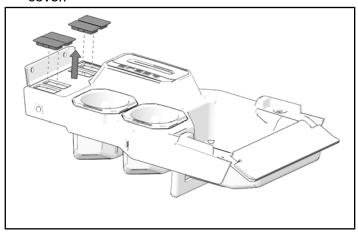
16. Trim foam seal and plastic rib on bottom of shift handle cover as needed to create clearance for main harness.
