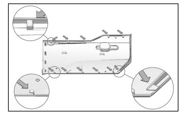
2. The filler panel for the rear doors has six engagement points. The lower rear corner of the panel fits over a tab on the door. The other five tabs engage with the main trim panel on the door.
