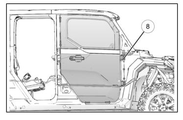
After door is properly positioned, check engagement with the striker. Adjust striker up or down as needed for proper latching. If door does not seal or rattles when latched, adjust striker inward. If door is diffcult to open, adjust striker outward. Remove striker cover to access striker screws.
