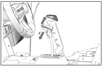
2. Remove screw from inside knob base. Remove knob base.
