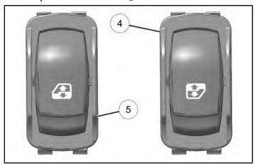
19. Connect four switches (4) to harness connectors. Push switches into openings in shift handle cover until switches lock into place.
