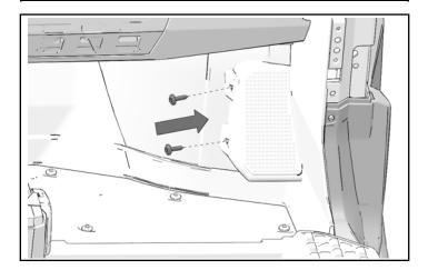
7. Install five push-pin rivets in front door opening.
