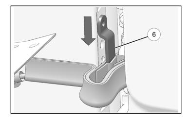
5. Install two screws ① to attach bracket ⑥ to A-pillar. Torque bracket screws to specification.
