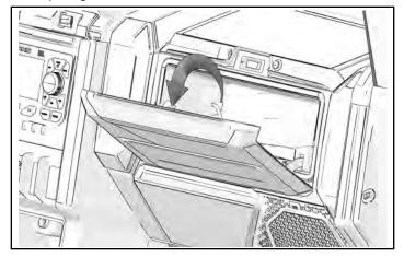
5. Remove and keep five screws (A) and washers at front of dash cover.
