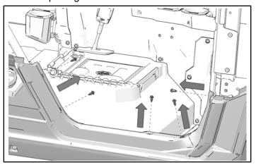
4. Remove and keep two screws from side of foothold in front of passenger seat area.
