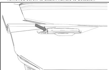
7. Push previously removed cover into place over the actuator.
