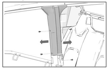
2. Remove and keep two screws from inside panel.
