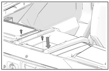
3. If vehicle is equipped with tip-out windshield. Install base, three screws, and washers. Torque screws to specification.
