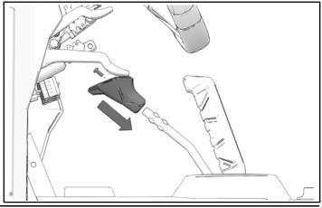
23. Install shift handle knob cap. Torque kept screw to specification.
