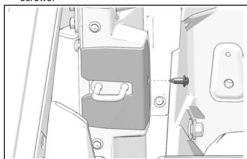
3. When finished adjusting the striker, torque striker screws to specification. Replace cover.
