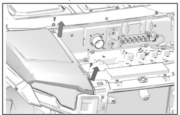
3. Pull fender outward to disengage upper tabs.
