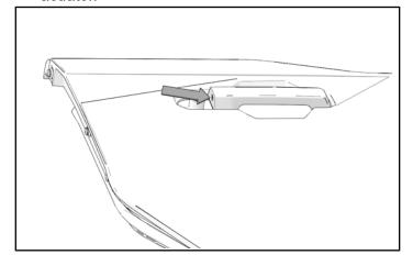
4. Lift handle away from actuator and pull backwards to remove handle. Keep handle for later installation.
