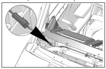
2. Put front of dash cover in position and set into place. Make sure center of dash is placed in slots on vehicle.
