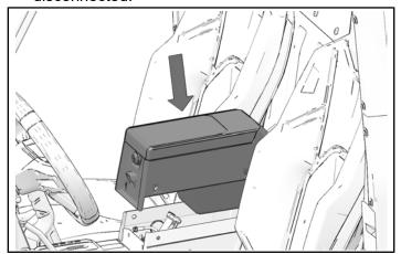
2. Install six push-pin rivets to attach center console.
