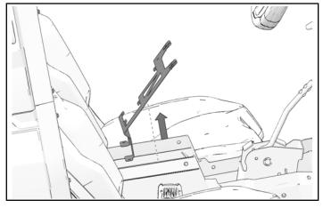
8. Install two U-clips (3) at top of bracket (6).
