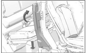
2. Install six push pin rivets.
