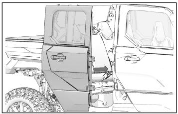
2. Loosely install four hinge screws  $\widehat{O}$ .
