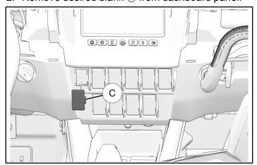
3. Feed light bar switch connector **1A** (from light bar harness ①) through opening in dash towards dashboard panel.
