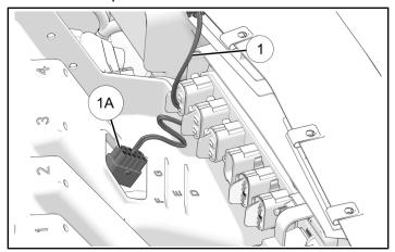
Install light bar switch ② from front in desired location. Plug connector 1A from light bar Harness
