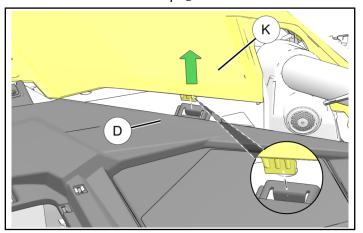
7. Carefully keep panels ① and ⑥ up and away from tabs and remove dashboard top ⑩ by tilting rear section up and pulling out toward rear.
