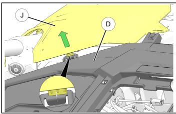
6. Carefully lift edge of right front fender (®) to release tab from dashboard top (®) as shown.
