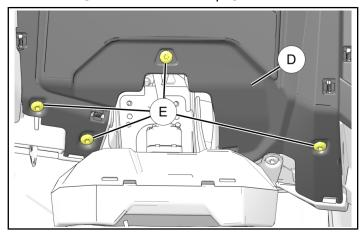
4. On front of vehicle, near rear edge of center hood panel opening, remove and retain two screws (§ from dashboard top (D). Remove and retain two pushpin rivets (H) from front side panels.
