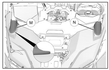
4. Reinstall two retained screws (a) into front edge of dashboard top (b) and two retained pushpin rivets
