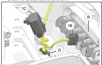
6. Route harness along top edge of firewall as shown, secure with attached clips ① to firewall. Positive (1D) and Ground (1E) connectors should be close to roll cage base.
