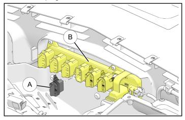
2. Remove desired blank © from dashboard panel.
