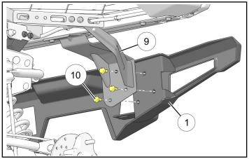
6. Torque all M8 screws ()(8)(10) to specification.
