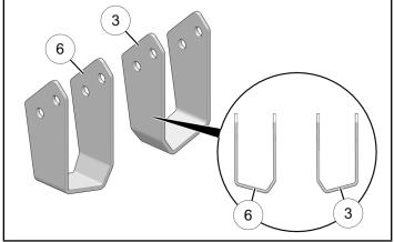
b. Install LH limiter bracket (6) to bed frame using two each screws (7), spacers (5), and nuts (4).
