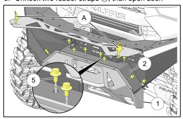
6. Loosely install mid bumper ② to lower bumper ① using ten screws ③.
