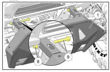
2. Install bottom of lower bumper ① to chassis using screw ⑦ and nut ⑧. Repeat for opposite side.
