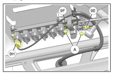
2. Torque two nuts (A) to specification, then reinstall red boot over post **BAT** +.
