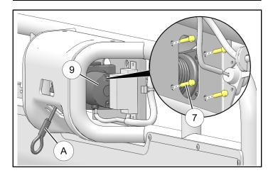
2. Install contactor 9A to frame using two each screws ① and nuts ③. Tighten screws.
