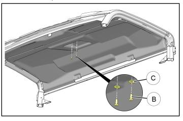
d. Carefully pull LH and RH edges of liner from between ROPS and roof seal, then remove rear edge of liner from roof support channel ①.
