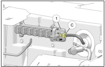
Install "T-BLOCK (B+)" battery cable to terminal block stud identified as "BAT +", then reinstall nut B. Torque nut to specification, then reposition red boot over stud.
