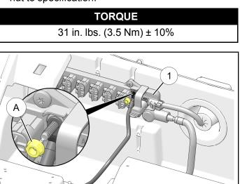
5. Reconnect accessory harness connectors to new terminal block ①.
