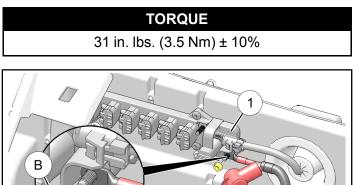
4. Install chassis ground cable to terminal block stud identified as "**BAT** –", then reinstall nut (A). Torque nut to specification.
