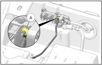
6. Slide red boot along **"T-BLOCK (B+)"** battery cable, remove nut **(B)** from terminal block stud identified as **"BAT +"**, then detach battery cable. Retain nut.
