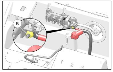
7. Detach harness connector © from terminal block connector identified as "ACC".
