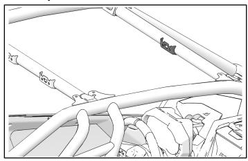
3. Align rearview mirror mount ① with U-clips ③ and install with two screws ②.
