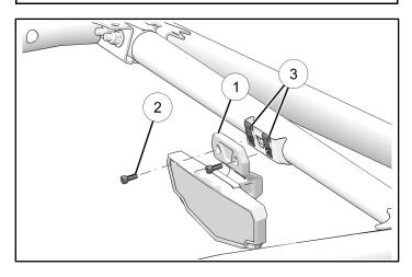
2. Snap two U-clips 3 onto bracket.
