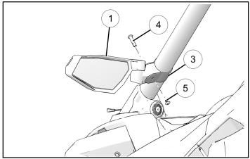
Position mirror at eye level when seated in vehicle. Use torx <sup>®</sup> to hold binding post receiver immobile, then tighten binding screw (5) to specification.
