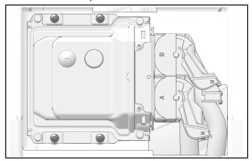
3. Lift levers up to disengage connectors.
