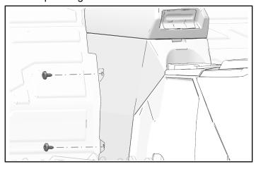
7. Remove center console storage compartment from vehicle.
