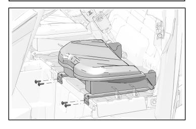
Position backrest assembly into seat base and lean back until headrest engages with receiver tube.
