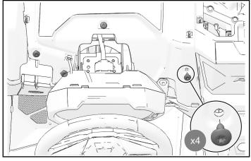
7. Open glove box lid and reinstall storage compartment. Install four retained dashboard fasteners around glove box opening.
