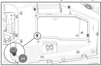
3. Remove and keep three front dashboard fasteners around glove box opening.
