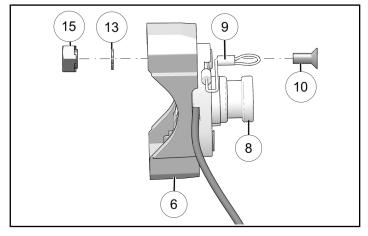
2. Each clamp comes with two sets of rubber collar inserts. Select the set designed to be used on ROPS ranging from 1-3/8 in. to 2 in. diameter. Install rubber collar insert ① into each clamp collar.
