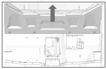
2. Install four close-off fasteners. Torque fasteners to specification.
