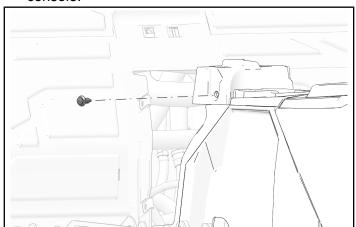
2. Remove and keep eight center console fasteners from passenger's side.
