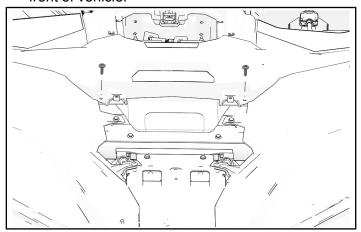
6. Remove and keep two push-pin rivets from front side hood panels.
