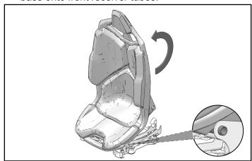
2. Lower seat onto rear receiver tubes.
