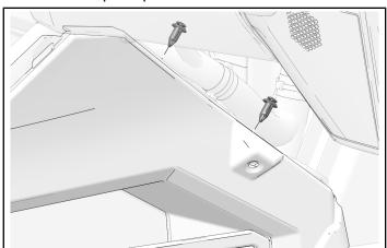
3. Install passenger side panel with eight retained center console fasteners and one push-pin rivet.
