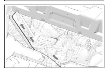
8. Install rear audio harness along horizontal chassis tube, behind upper close-off panel, with cable ties (sold separately), as shown.
