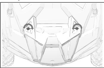
2. Install dashboard with four dashboard fasteners.
