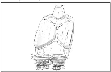
2. Tilt seat assembly forward and pull back slightly to disengage from receiver tube and remove seat from vehicle.
