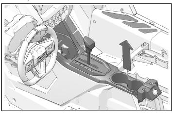
2. Install two push-pin rivets .
