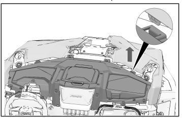
9. Carefully keep panels up-and-away from tabs and remove dashboard top by tilting rear section up and pulling out toward rear.
