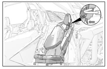
2. Remove and keep four seat bracket fasteners. Remove seat from rear seat panel.
