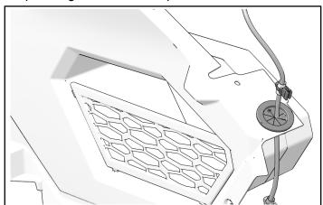
2. Loosely reinstall passenger-side console panel and begin routing audio harness to accessory mounting panel. Secure to vehicle with edge clips 3D.
