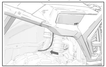
5. Install rear audio harness to chassis electrical harness in tunnel with cable ties (sold separately).
