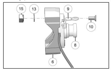
Each clamp comes with two sets of rubber collar inserts. Select the set designed to be used on ROPS ranging from 1-3/8 in. to 2 in. diameter. Install rubber collar insert ① into each clamp collar.
