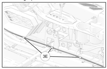
6. Route audio harness along chassis harness, behind rear close-off panel. Use cable ties at taped locations 3E or routing clips 3F.
