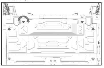
2. Turn each knob 1/4 to disengage and remove bottom close-off panel.
