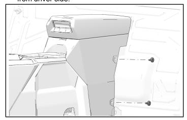
6. Remove and keep two center console fasteners from passenger side.
