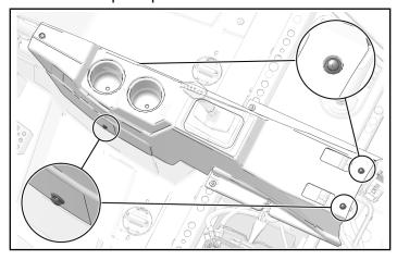
4. Pull shifter boot and seat belt buckle boots through center console openings and make sure they are properly seated.
