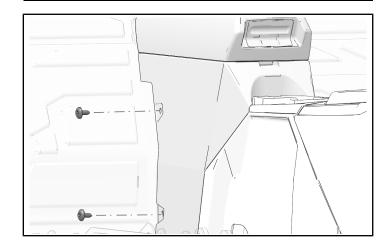
3. Install console storage compartment with two retained center console fasteners from driver side.
