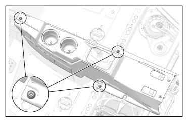
3. Install four push-pin rivets.
