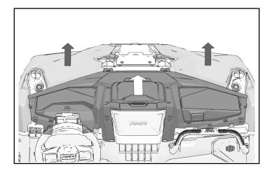
Make sure tabs on panels are aligned in slots on dashboard top. (Passenger-side panel shown; driver-side panel similar.)
