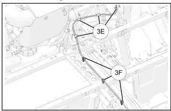
7. Route audio harness along chassis harness, behind rear close-off panel. Use four cable ties at taped locations 3E.
