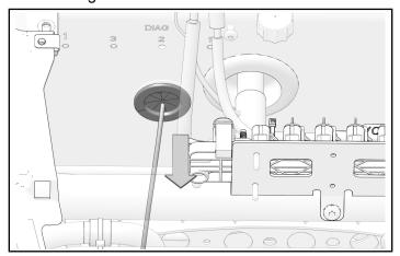
4. Put connectors through tunnel opening.
