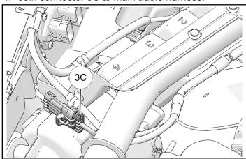
5. Route harness along tunnel, securing with routing clips.
