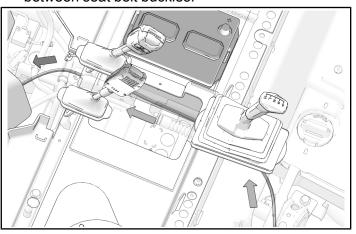
7. Pull harness out from lower close-off and install to frame tube with cable ties (sold separately).
