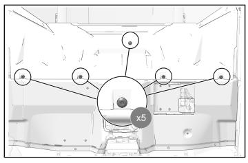
4. Install four push-pin rivets.
