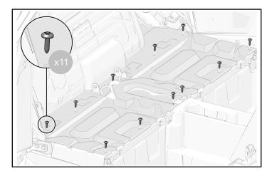
2. Reinstall one push-pin rivet in right-rear of seat panel.
