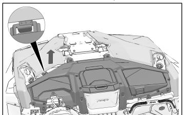
8. Carefully lift edge of right front hood panel to release tab from dashboard top as shown.
