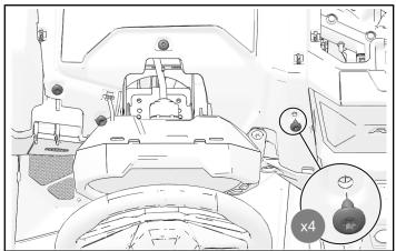
5. Remove and keep two dashboard fasteners from front of vehicle.
