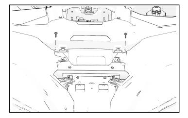
5. Install hood panels to vehicle with two retained push-pin rivets
