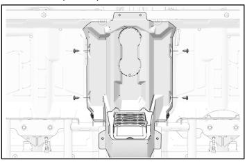
3. Remove and keep four push-pin rivets.
