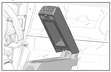
2. Turn each knob 1/4 to disengage from center console panel.
