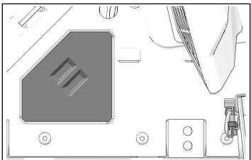
11. Route audio harness along chassis harness, behind close-off panel. Use three cable ties at taped locations 3E.
