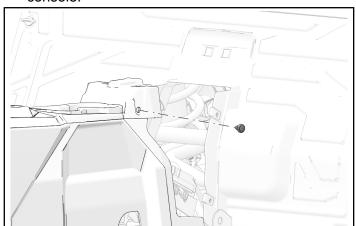
2. Remove and keep eight center console fasteners from driver's side.
