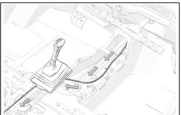
6. Install harness around shifter assembly and between seat belt buckles.
