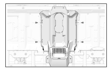
4. Install to front-center console with two center console top fasteners (longer).
