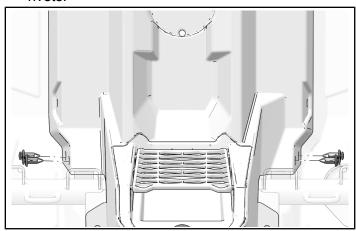
3. Install sides with four center console side fasteners (shorter).
