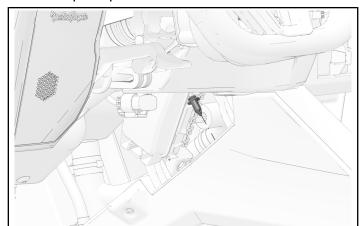
2. Install retained push-pin rivet and fuse block fastener. Torque two fuse block fasteners to specification.
