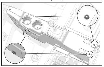
2. Remove and keep three console fasteners.
