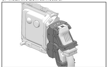
6. Install ECM to close-off panel with four retained fasteners. Torque fasteners until fully seated.
