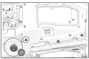
Tilt steering wheel down. Remove and keep four dashboard fasteners from dashboard surrounding steering wheel.
