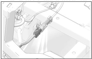
3. Put two rear speaker pod connectors through firewall grommet toward front of vehicle.
