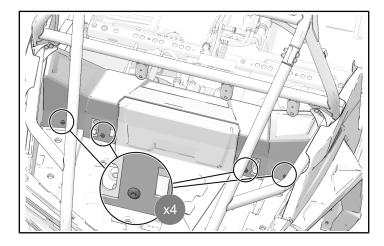
3. Install five close-off fasteners. Torque fasteners to specification.
