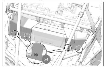
7. Lift upper close-off panel to remove lower close-off panel.
