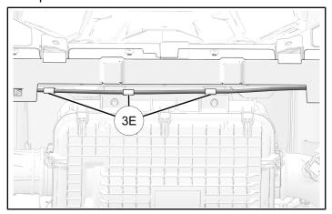
12. Attach harness to vehicle frame with two edge clips 3D.
