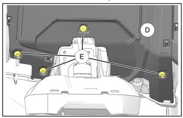
4. On front of vehicle, near rear edge of center hood panel opening, remove and retain two screws © from dashboard top ①. Remove and retain two pushpin rivets ® from front side panels.
