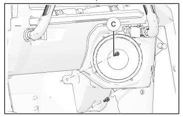
5. Remove and retain two push-pin rivets to ease speaker removal.
