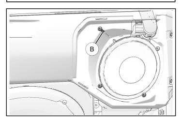
11. Install bottom of subwoofer with two mounting fasteners (4).
