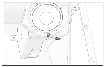
6. Maneuver speaker out from under dashboard. Carefully set aside for reinstallation.
