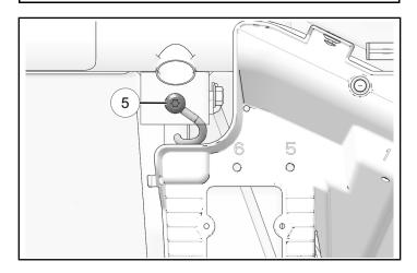
7. Tilt right-hand driver assembly up-and-into installed position. Ensure driver cable routes upwards into under-dashboard.
