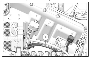
2. Install fuse relay 1A onto accessory mounting panel at location marked 4.
