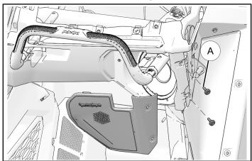
3. Remove and retain four fasteners © to uninstall speaker from dashboard panel.
