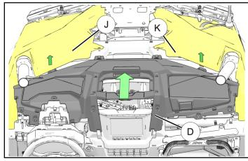
2. Ensure that tabs on panels ① and ® are aligned in slots on dashboard top ⑩. (Panel ® shown; panel ① similar.)
