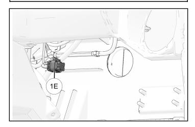
4. Rotate subwoofer assembly 90°, with rear of subwoofer directed towards center of vehicle, and begin positioning subwoofer beneath dashboard.
