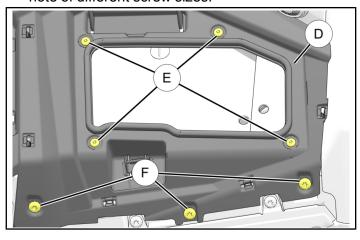
3. Tilt steering wheel down. Remove and retain four screws (£) from dashboard top (D).
