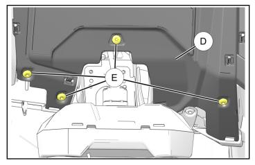
6. Open glove box lid and reinstall storage compartment. Install four retained screws (E) around glove box opening and three retained screws (F) in front of dashboard top (D). Torque screws to specification.
