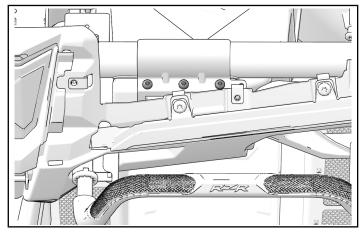
6. Remove ground terminal fastener (5) and reinstall with subwoofer ground terminal attached.
