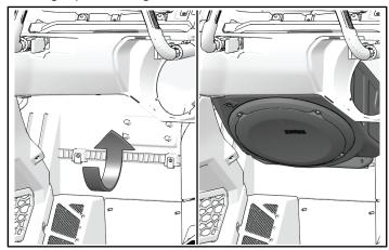
Reinstall subwoofer bracket to subwoofer, ensuring bracket hooks onto vehicle frame. Tighten subwoofer bracket fasteners to specification.
