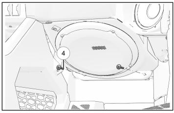
12. Reinstall two dashboard panel fasteners.
