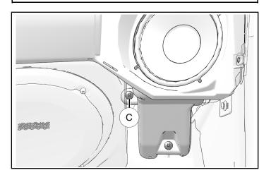
10. Install speaker to dashboard panel with four fasteners ③.
