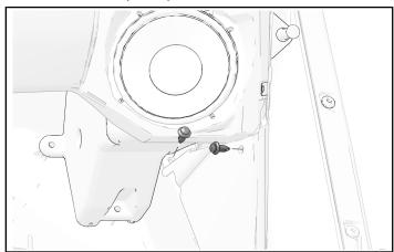
9. Install right-hand speaker with two retained speaker fasteners ©.
