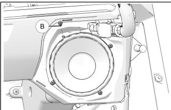
4. Remove and retain two speaker fasteners ©.
