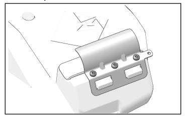
2. Install two U-clips 3 onto front cab panel.
