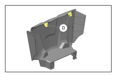
4. Install new winch cover ① by inserting two upper tabs, then installing two screws ②.
