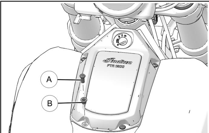
2. Tilt center console up to remove from tank cover.
