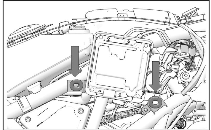
3. Place each tank cover on alignment bracket. Ensure each alignment tab is seated within corresponding tank cover hole.
