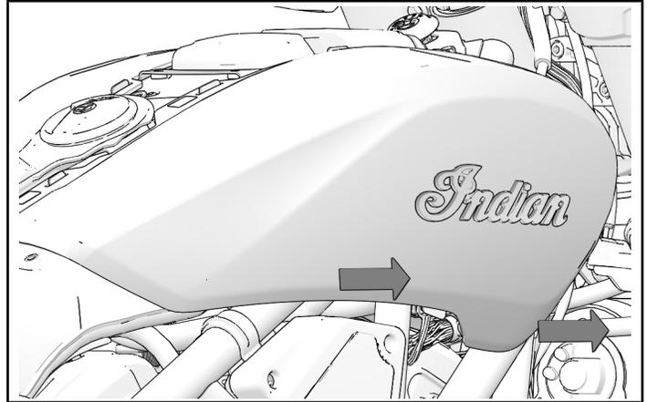
5. Pull each cover directly upward and free of alignment tabs.
