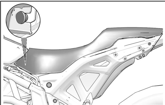
4. Secure rear of seat with two retained seat fasteners (B).
