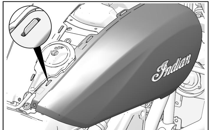
4. Firmly push lower tank cover into grommets. Ensure both tank cover rivets are firmly seated and grommet has not been pushed through bracket.
