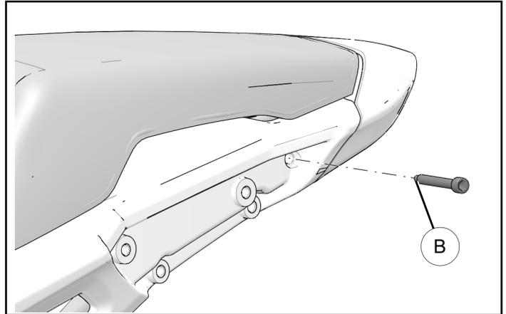
5. Install each passenger handle with two retained handle fasteners (A).
