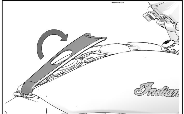
8. Reinstall tank bezel with four retained bezel fasteners ① and four retained compression limiters ②.
