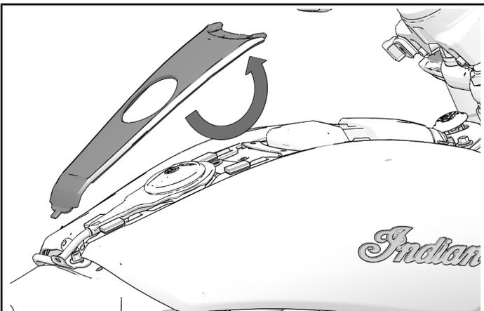
3. Remove and retain two tank cover fasteners (C) from rear-end of tank covers.
