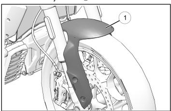
2. Loosely install fender ① with four mud guard fasteners ② and four washers ③, before torquing hardware.
