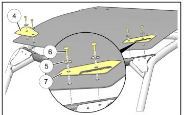
6. Loosely install rear of roof to brackets (8) using four each screws (6) and washers (5).
