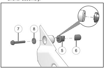
2. Align three wedge lock anchor assemblies of rock slider within vehicle chassis. Ensure each anchor assembly is fully seated before torquing.
