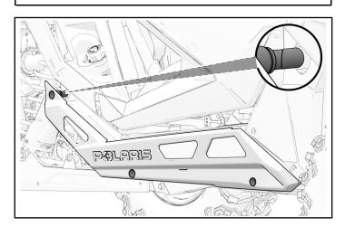
3. Firmly push end caps ③ and ④ (*Premium Rock Sliders Kit* only) into each mounting location.
