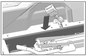
4. Remove and discard nut ® from buckle connecting bolt. Disconnect speed-regulator connector. Remove and discard seat belt buckle.
