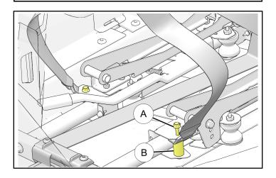
4. Install rear harness brackets onto rear seat base with one screw ① and one nut ⑧ per side.
