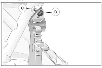
4. Remove and discard on nut <sup>®</sup> from seat belt retractor.
