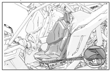
2. Tilt seat assembly forward and pull back slightly to disengage from receiver tube. Remove seat from vehicle.
