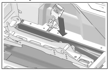
6. Remove and discard bolt ©. Remove and discard seat belt buckle.
