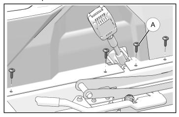
2. Remove and retain four screws (A) from RH center console panel.
