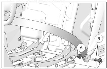
3. Remove and discard one nut © and one bolt ® from upper seat belt bracket.
