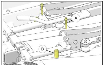
2. Stack harness brackets atop each spacer ® groove.
