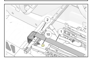
Install front harness guide ③ onto retractor bracket
