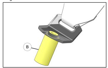
3. Install harness bracket / spacer ® assemblies with two retained screws ⓐ, within seat roller brackets.
