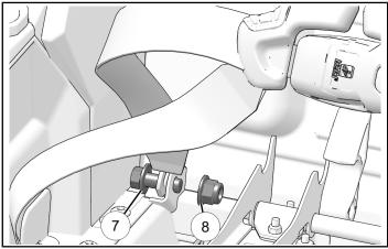
5. Install shoulder harness brackets with two bolts ① and two nuts (8).
