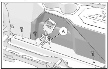
3. Carefully push center console panel and underseat panel down to access connecting hardware.
