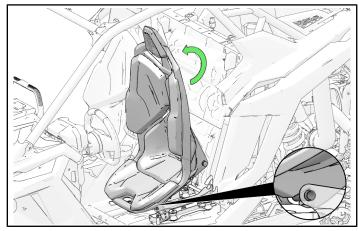
2. Lower seat onto rear receiver tubes.
