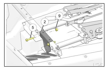
2. Mount retractor/harness assembly ① onto retractor bracket ② with one nut ⑩.
