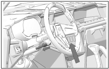
2. Lift upward on front driver seat latch lever located on bottom backside of seat.
