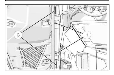
3. Push door inwards while attempting to center door in ROPS/chassis opening. Hold door in place, then observe gap between door window ① and ROPS/chassis (around entire perimeter of door).
