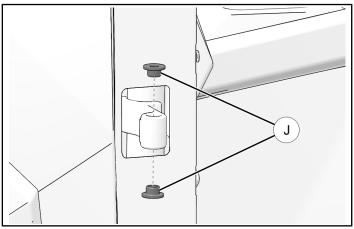
3. Insert new bushing <sup>(6)</sup> from top down into all vehicle-side hinges.
