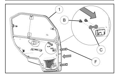
2. Position new door ① so door-side hinge pin holes align with vehicle-side hinge pin holes.
