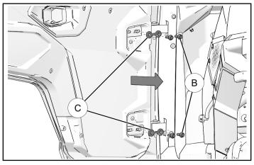
3. Slide door assembly off door-side hinges.
