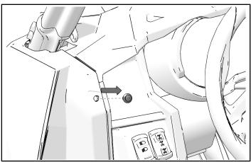
2. Assemble outboard (2) and inboard (3) A-pillar trim with two screws (5). Do not overtighten screws.
