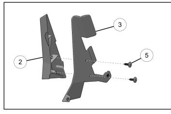
3. Install A-pillar trim with screw ④ and retained push-pin rivet.
