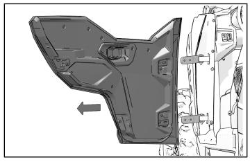
Remove two screws D, then remove striker plate
