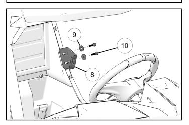
Install striker pin ① and conical spring washer ② to striker bracket ⑧ using nut ⑧. Make sure cupped side of washer is towards striker bracket. Position striker in middle of adjustment slot.
