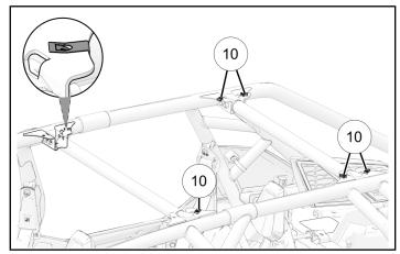
5. Install four U-nuts 10 onto ROPS, as shown.
