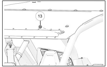
12. Verify torque specification of roof fasteners. Torque may change due to foam compression.
