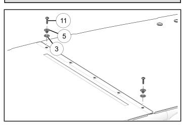
10. Install inside of front roof panel to rear roof panel with three fasteners 1, three spacers 5, and three washers 4
