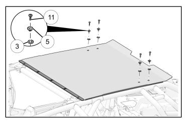
7. Install front roof panel with four fasteners (1), four spacers (5), and four washers (3).
