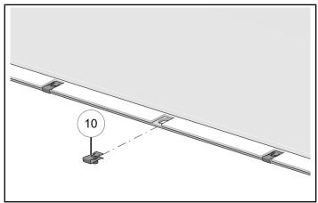
4. Install six U-nuts 10 onto ROPS, as shown.
