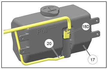
b. Join connector 18D on power harness (8) to mating connector on washer bottle pump.
