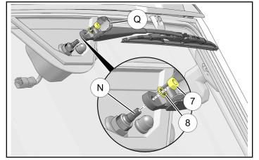
8. Hold wiper blade/arm assembly parallel to the top of the windshield while applying torque to prevent damage to wiper motor. Torque nut to specification.
