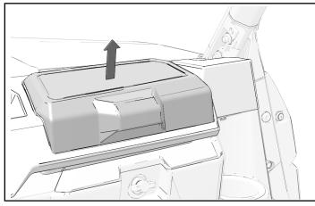
g. Remove two push-pin rivets from storage compartment location on dashboard. Retain rivets.
