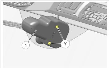
c. Install bracket <sup>(A)</sup> (with attached mirror assembly) to motor assembly <sup>(1)</sup> using two #14 X 3/4 High/Low screws <sup>(6)</sup>.
