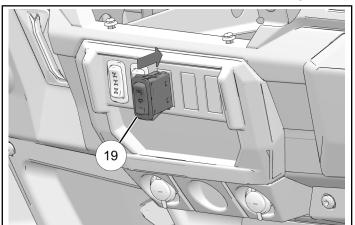
g. Reaching through cupholder cutout, join connector 18E on power harness (18) to switch (19).
