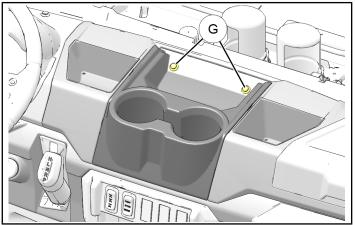
b. Remove six push pin rivets ① along forward edge of dash.
