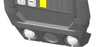
f. Install switch (19) in control panel opening.
