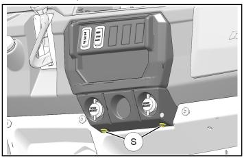
c. Rotate bottom of control panel rearward, disengaging two side tabs ①, then drop two upper tabs ① out of slots in main dash panel.
