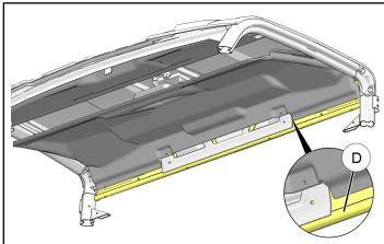
e. Remove front roof liner by removing two each screws (£) and washers (£). Retain hardware.
