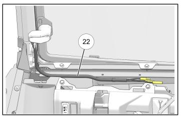
MATCHING WIRE COLORS, join bullet connectors 22A–22D on ROPS harness <sup>(2)</sup> to mating bullet connectors 18G–18K on power harness <sup>(8)</sup>.
