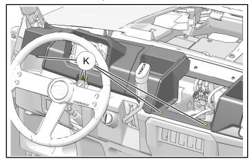
d. Open door to upper storage compartment. Remove three push pin rivets ① from RH side of dash: two inside storage compartment and one on underside of dash above cupholder.
