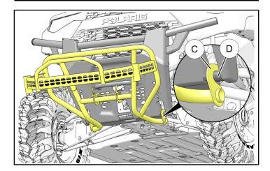
4. Lift bumper upwards until upper hook assembly (B) can rotate over upper bumper tube (E).
