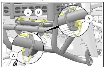
5. Secure upper hook assembly ® to upper hook brackets using two wire lock pins (A).
