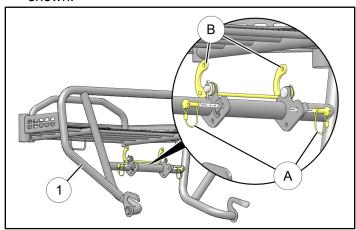
3. Insert two lower hooks © over lower bumper tube D.
