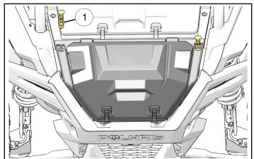
5. Lock & Ride<sup>®</sup> assemblies ① may need adjustment. Tighten or loosen bottom nut depending on fitment.
