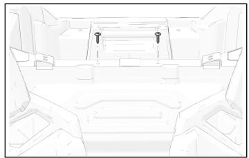
Install rear panel bracket ② with two retained fasteners. Ensure vertical part of bracket is facing rearward.
