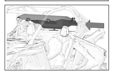
4. Carefully, position rear panel so that side clamps rest on vertical ROPS.
