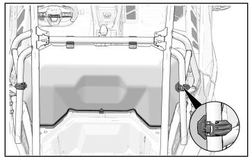
7. Press top clamps upward to engage beneath horizontal tube.
