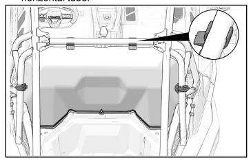
8. Secure rear panel to bracket with knob fastener
