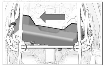
5. Compress seal to fit securely against body panel. Ensure mounting bracket is outside of rear panel.
