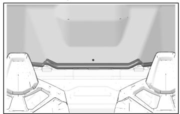
6. Press side clamps downward to engage on top of vertical tubes.
