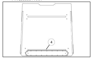
2. Install eight U-nuts ① onto ROPS, as shown. Convex part of each nut will fit into mounting hole of each mounting plate.
