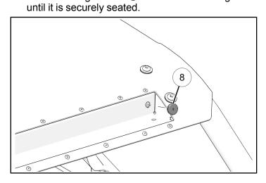
8. Verify torque specification of roof fasteners. Torque may change due to foam compression.
