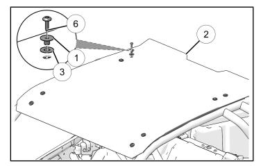
7. **P/N 2883961-XXX Only:** Push rubber grommet ® into harness routing hole
