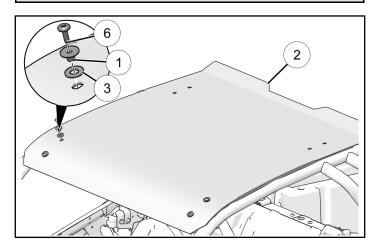
4. With front of roof panel ② secure to vehicle ROPS, begin to slowly pull roof panel ② back so that it molds to ROPS curvature.
