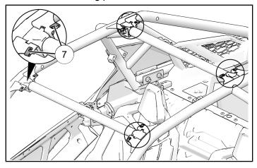
3. Install front of roof panel ② with four washers ③, four spacers ①, and four screws ⑥.
