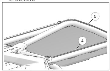
6. Secure rear of roof panel ② to ROPS with four washers ③, four spacers ①, and four fasteners ⑥.
