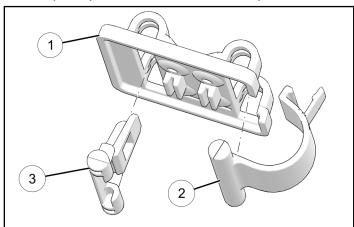
2. Test hoop ② and latch ③ movement to ensure both are fully installed.
