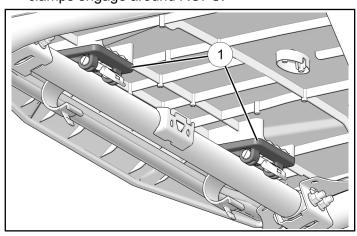
3. Wrap hoops ② around ROPS front cross-beam and secure with latch ③.
