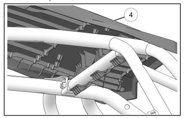
2. Rest clamp assemblies ① onto ROPS front crossbeam. Firmly push roof panel into place until clamps engage around ROPS.
