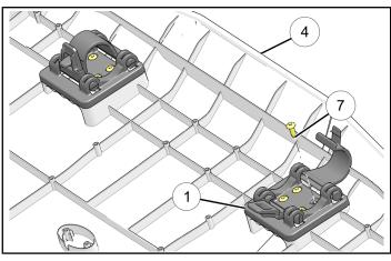
2. Slide two U-clips **(6)** onto roof panel **(4)**. Tabs on U-clips **(6)** will set within mounting holes of roof panel **(4)**.
