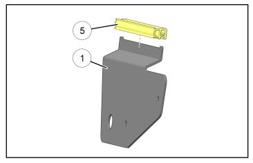
b. Install bumper ② to front side of bracket ① as shown.
