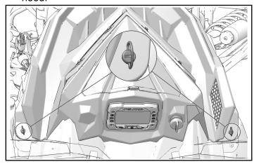
3. Slightly lift rear of hood and disconnect hood harness connector ① from main harness.
