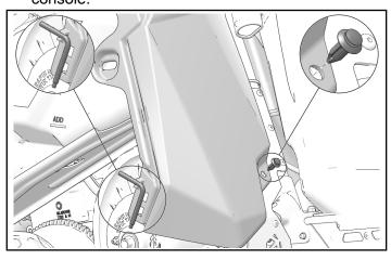
3. Install two dart clips on right side of console.
