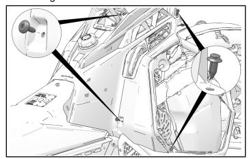
9. Remove fuel cap 1 and plastic fuel filler neck nut M.
