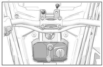
7. Remove and keep one push dart, two screws, and one clutch tool © from left side of console.
