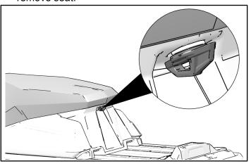
6. Remove and keep two push darts. Lift off switch panel.
