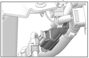
5. Use one cable tie ② to bundle extra length of RCA power wire and attach to main vehicle harness.
