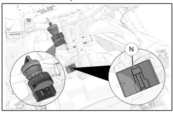
3. Reinstall plastic fuel filler neck nut M fuel cap L.
