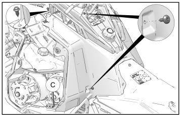
8. Remove and keep two push darts and two screws from right side of console.
