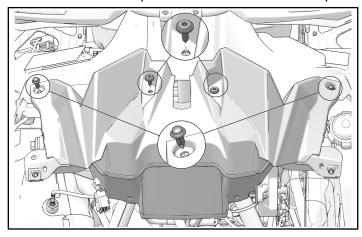
4. Lift off and set aside upper intake plenum.
