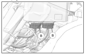
3. Remove and keep two screws and two dart clips.
