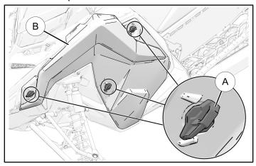
2. Turn the two 1/4 turn fasteners at rear corners of hood.
