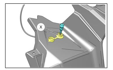
2. Push/pull remaining portion of plug into grommet until it is flush with the end, as shown.
