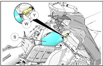
4. **Matryx models:** Connect RCA power wire connector to vehicle harness connector. Vehicle connector will be labelled "RCA plug."
