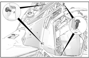
5. Install one push dart, two screws, and one clutch tool © on left side of console. Torque screws to specification.
